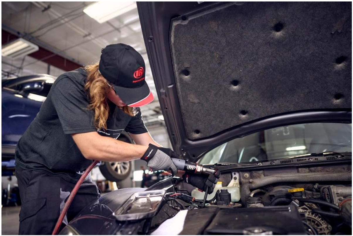
Figure 3: A mechanic utilizing the air ratchet wrench to work on an engine compartment, demonstrating typical use.
