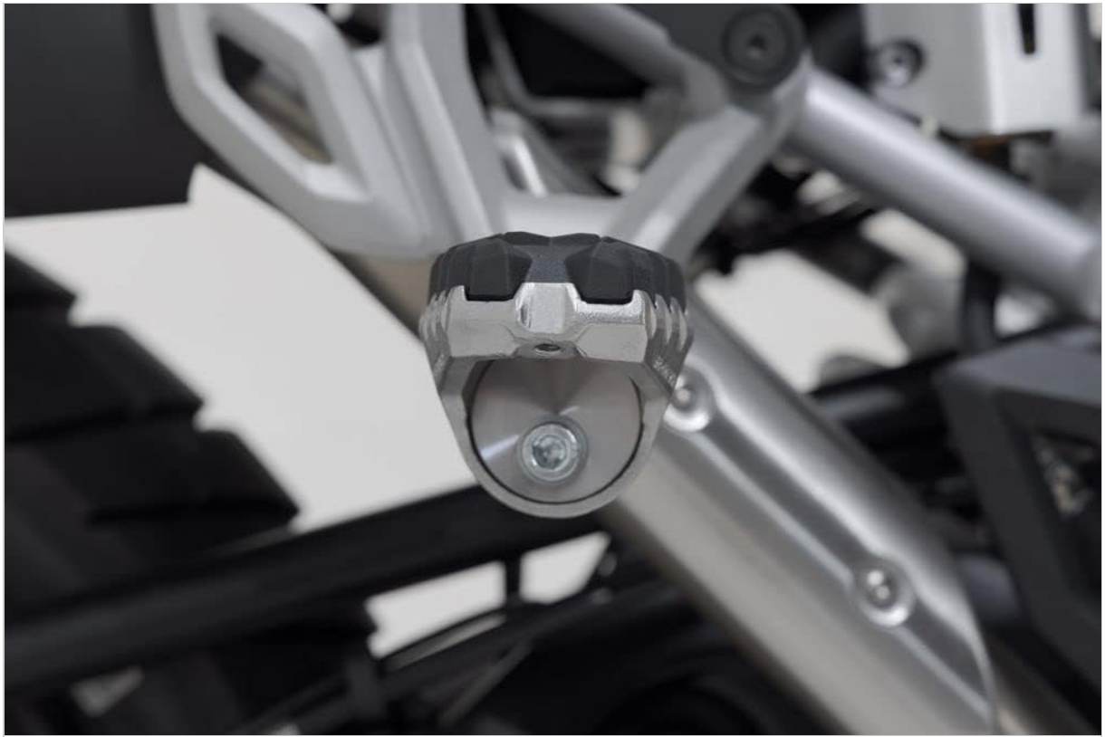
Figure 2: A direct front view of the SW-Motech footpeg, showcasing its sturdy design and the wide, textured surface for improved grip.
