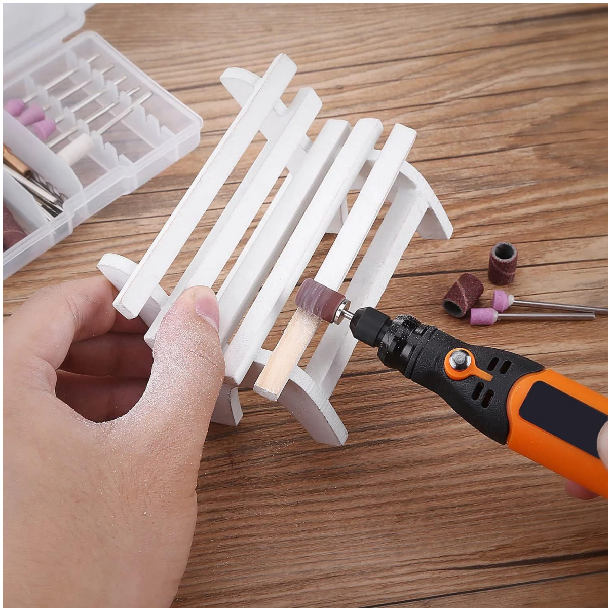
Image 4.2: The rotary tool in use for sanding a small wooden craft, demonstrating its application for finishing tasks.
