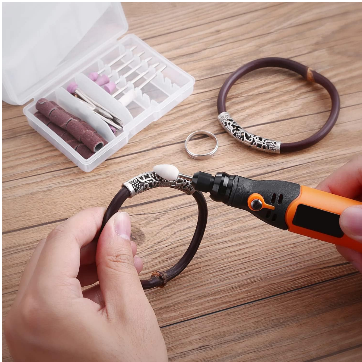
Image 4.3: The rotary tool being used for detailed work on a bracelet, showcasing its precision for engraving or fine adjustments.
