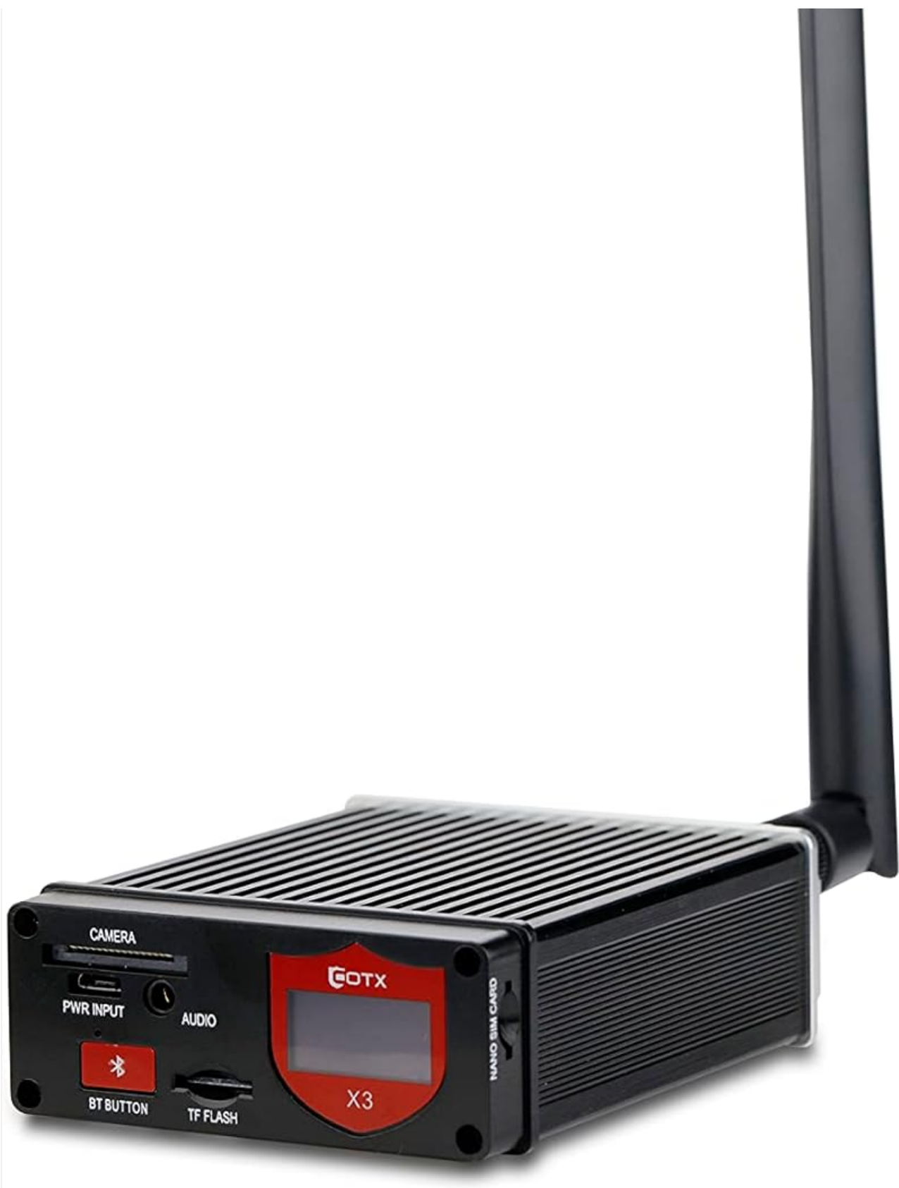
Figure 1: Front view of the COTX-X3 Indoor Full Helium Hotspot with its external LoRa antenna.
