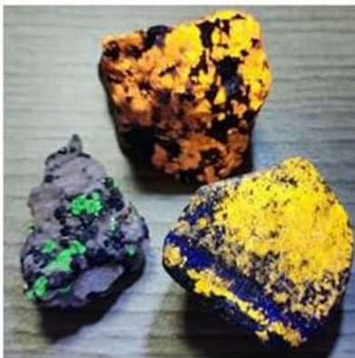
Figure 9: A visual comparison showing how minerals fluoresce more distinctly under 365nm UV light compared to 395nm UV light or normal light.
