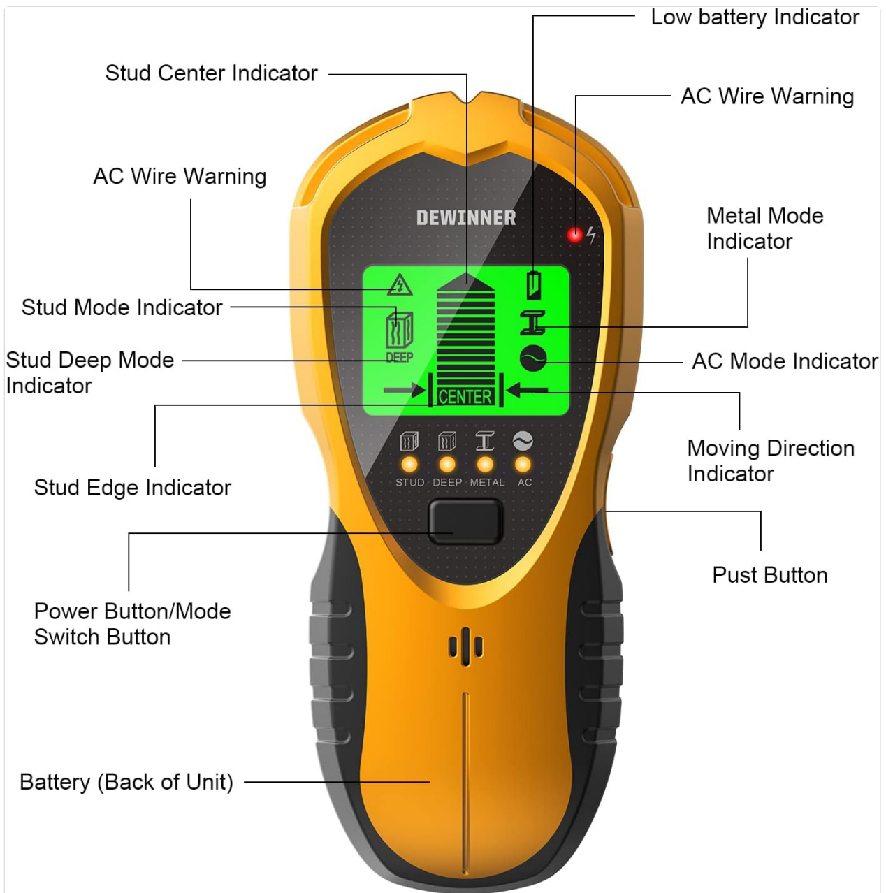
Figure 5: Labeled diagram of the DEWINNER Wall Detector's display and controls.
