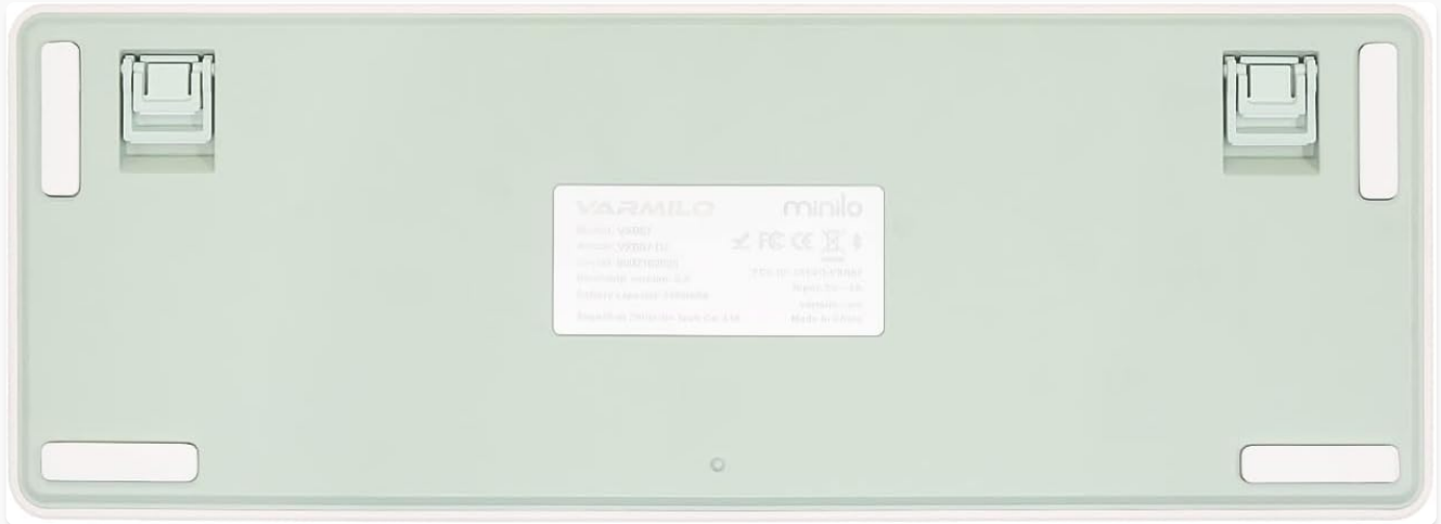
Figure 3: The underside of the Varmilo Minilo VXT67 keyboard, highlighting the mode switch for wired, 2.4GHz, and Bluetooth connections, along with the adjustable feet.
