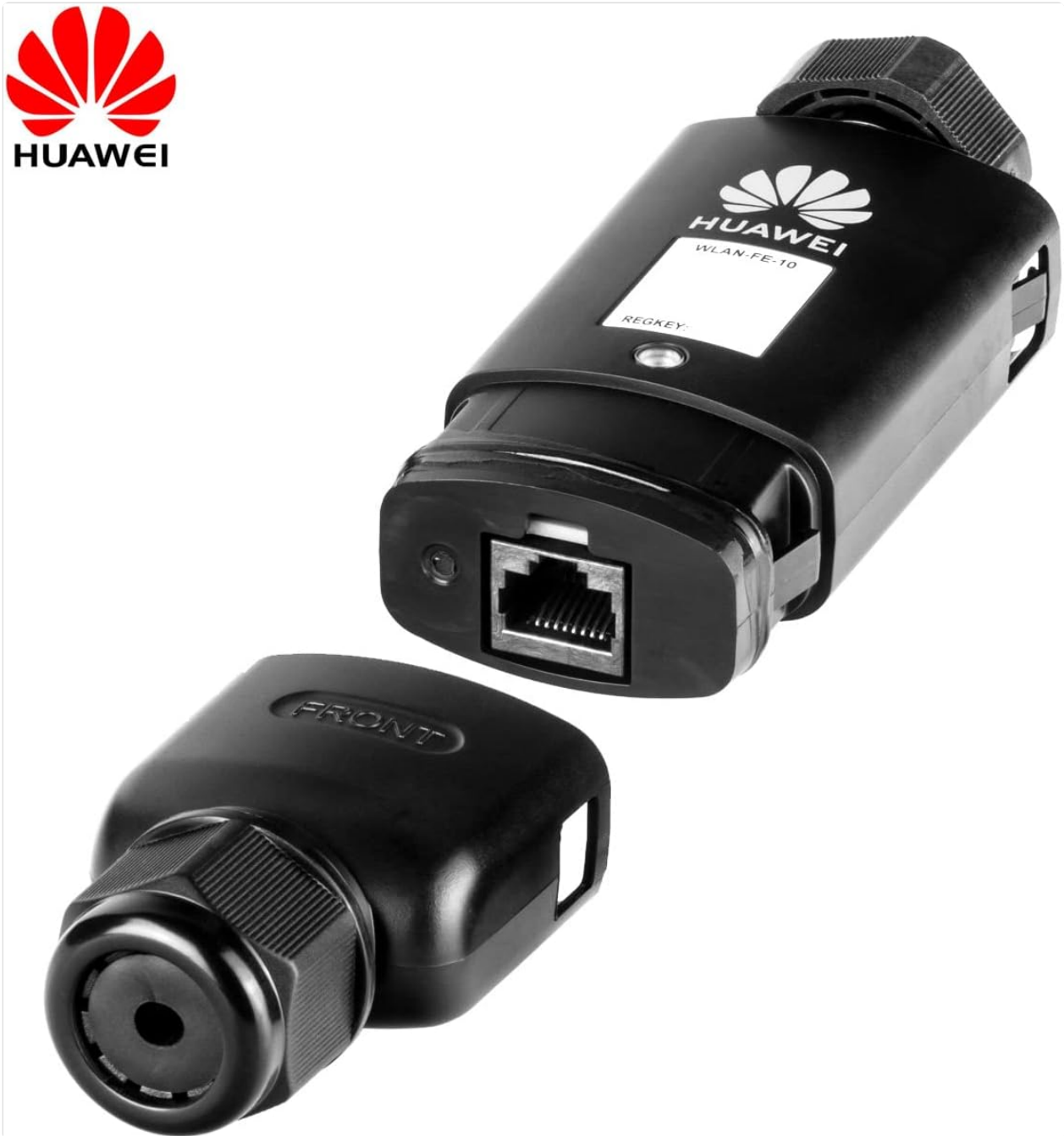
Figure 3: The Huawei Smart Dongle detached, showing the Ethernet port and USB connector, highlighting its modular design.
