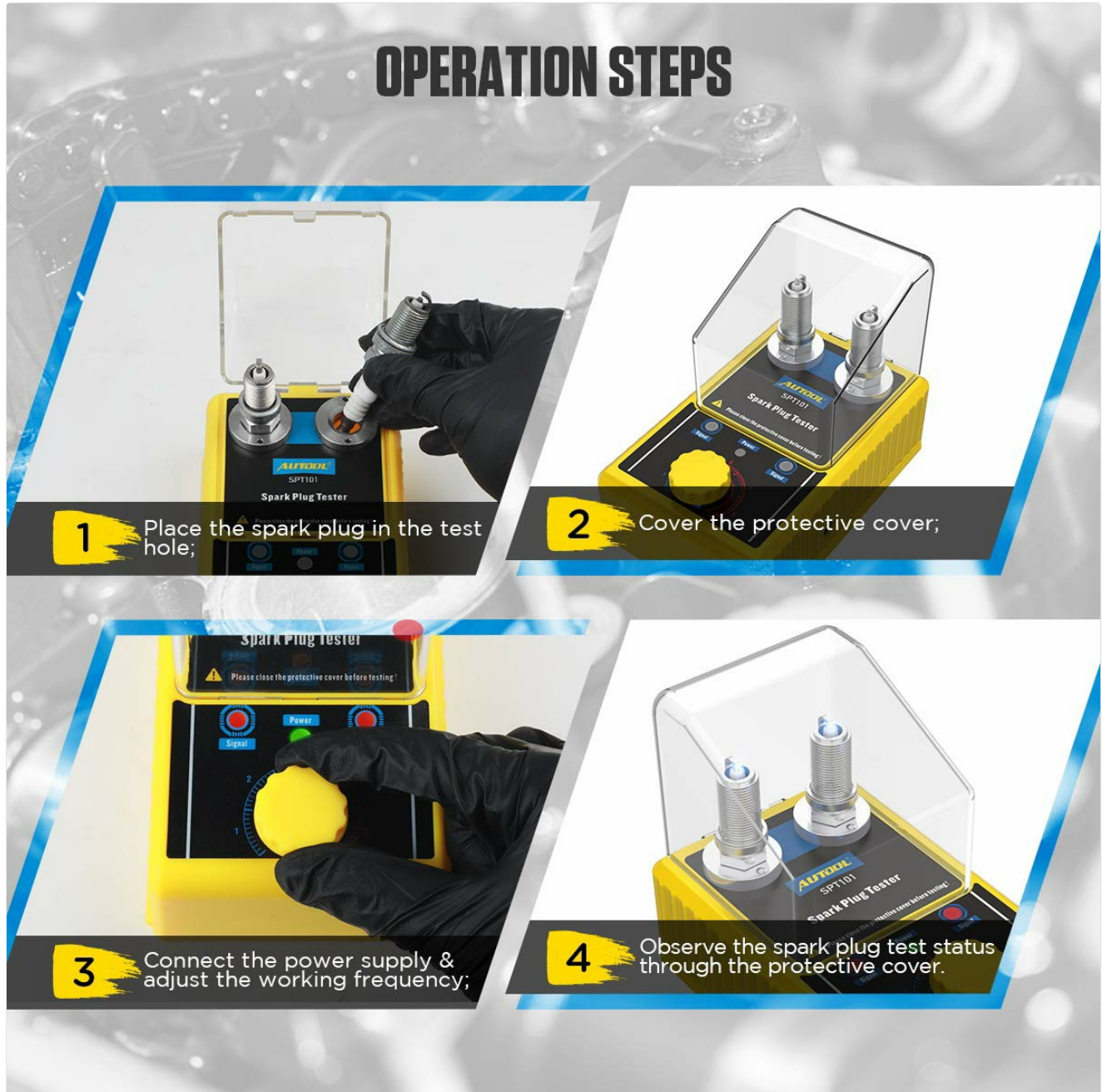
Image: A visual guide illustrating the four main operation steps: 1. Placing the spark plug, 2. Covering with the protective cover, 3. Connecting power and adjusting frequency, and 4. Observing the spark through the cover.
