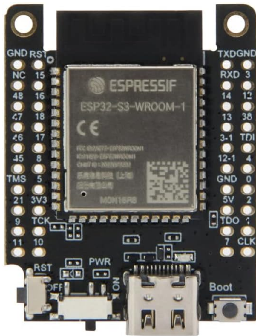
Figure 3.1: Front view of the LILYGO T7-S3 board, showing the ESP32-S3-WROOM-1 module, USB-C port, power switch, and boot button.
