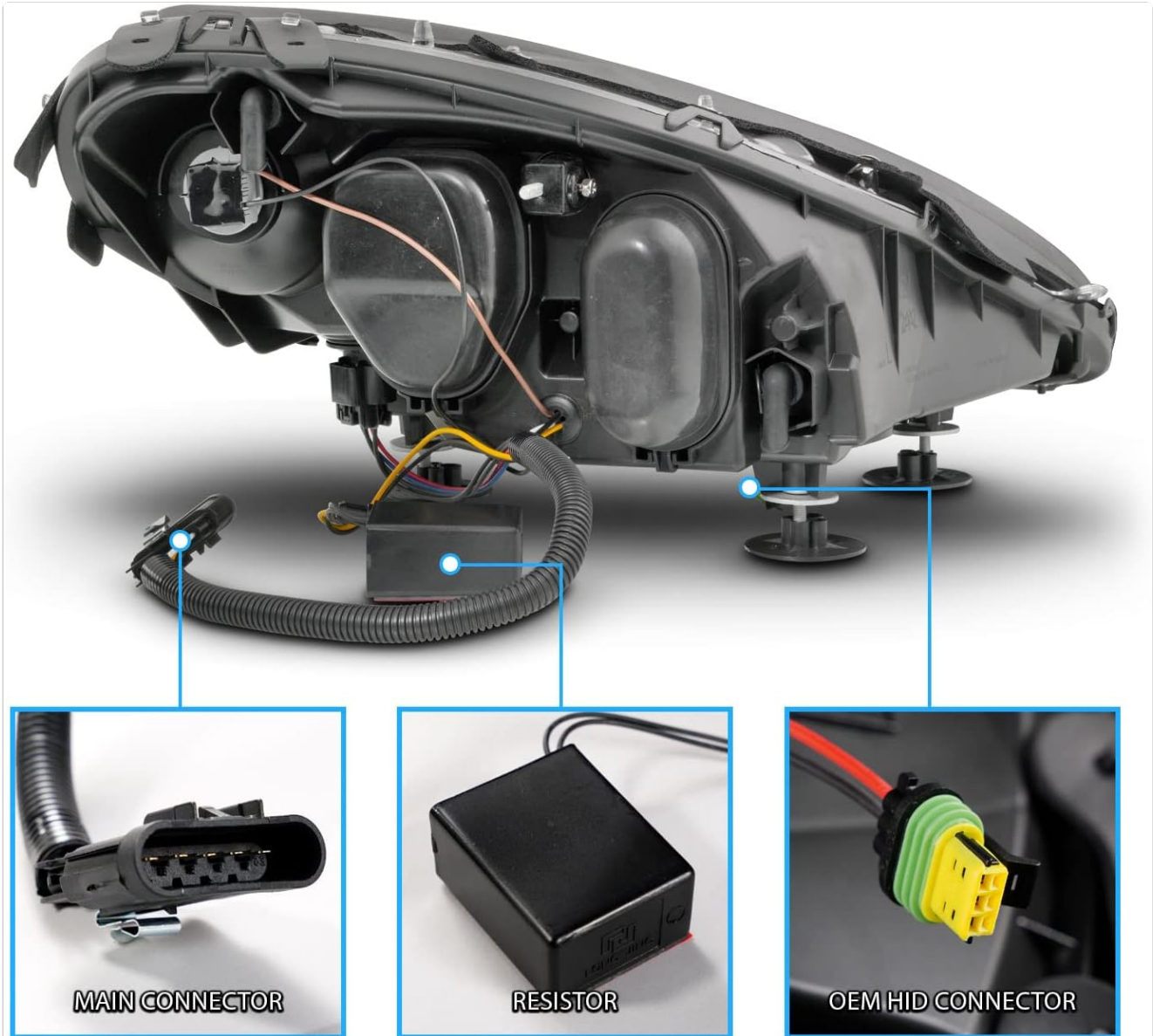
Figure 6: Rear view of the headlight assembly, illustrating the main connector, resistor, and OEM HID connector for wiring.
