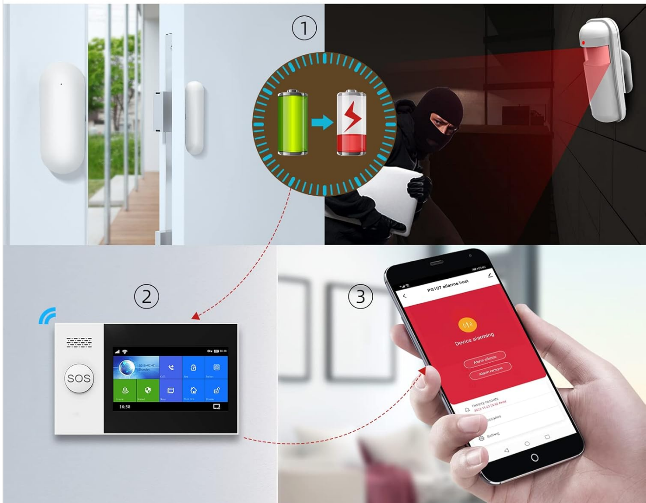
Figure 5.1: The system notifies you when wireless sensor batteries are running low.
