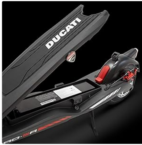
Figure 3: View of the battery compartment, indicating the location for charging.
