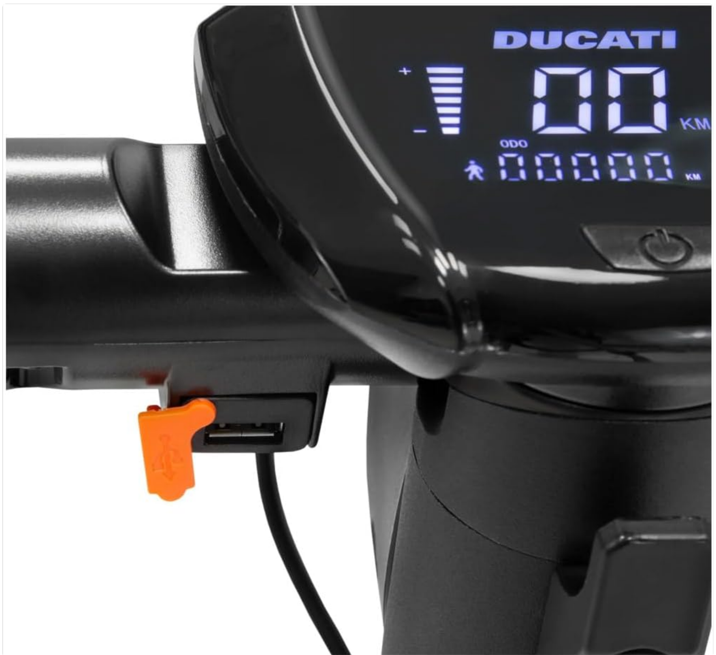
Figure 5: The scooter's digital display provides real-time information and includes a USB charging port.
