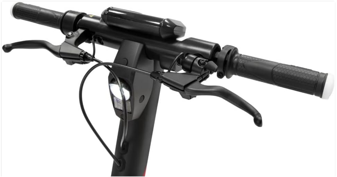
Figure 2: Detail of the handlebar assembly, showing brake levers and integrated controls.
