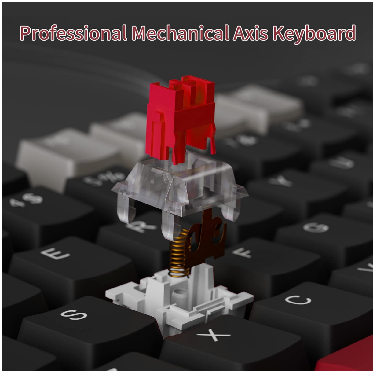
Detailed view of a red mechanical switch, highlighting the hot-swappable design.
