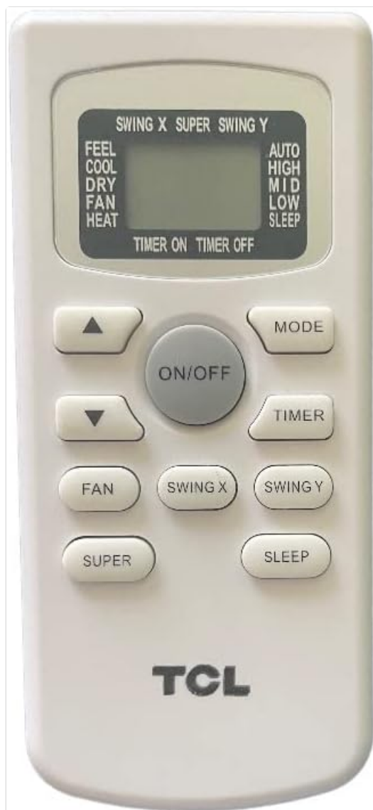
Figure 4.1: Front view of the remote control. Note: While the image displays a 'TCL' logo, this remote is compatible with Continental Minisplit CEDAC011MX as specified.
