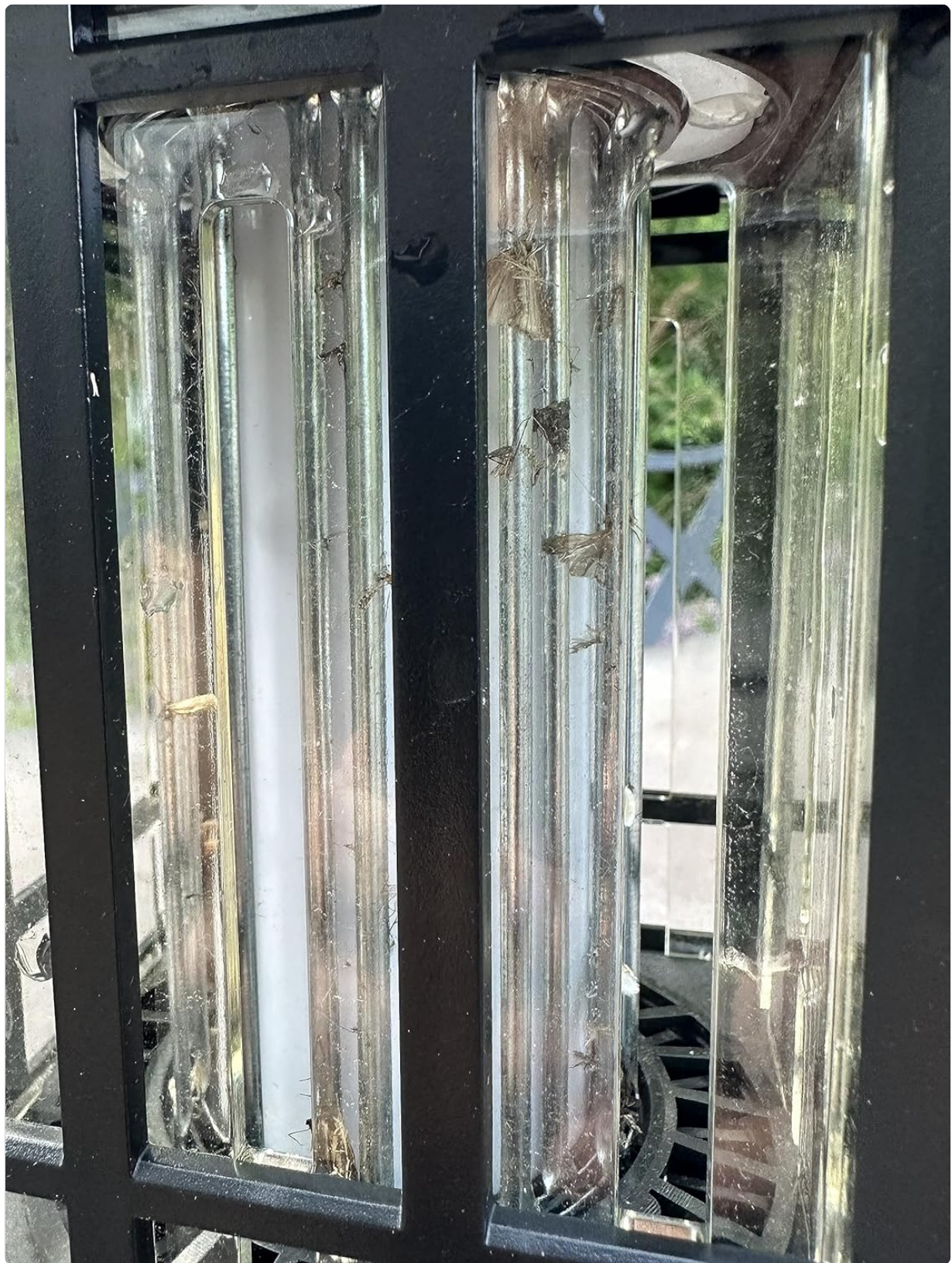
Figure 8: The zapping grid showing accumulated insect remains, indicating the need for cleaning.
