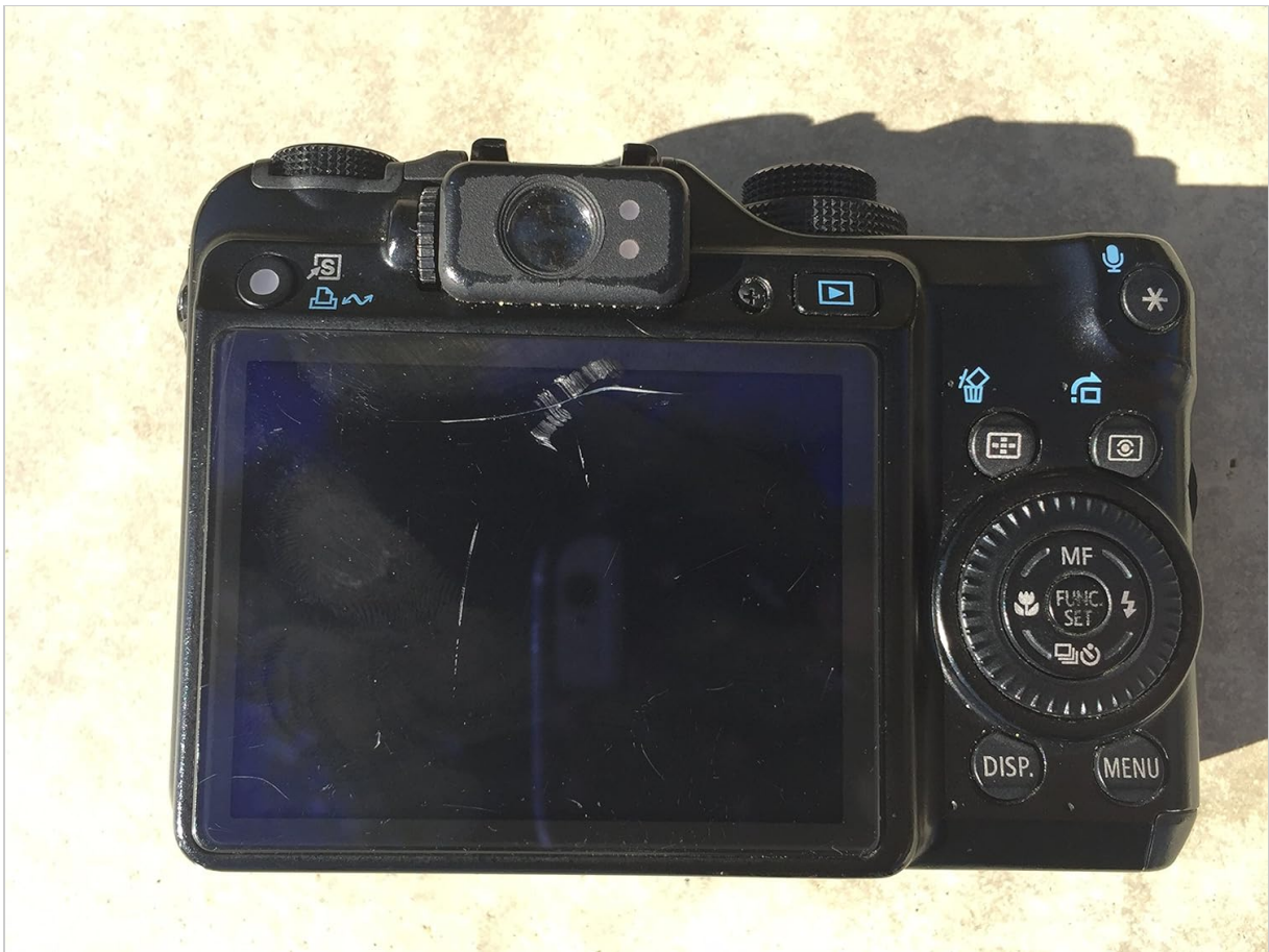
Image: Rear view of the Canon PowerShot G10 camera. This view displays the 3.0-inch PureColor LCD II screen, the multi-function controller, and various control buttons such as DISP, MENU, and the MF/FUNC.SET dial.
