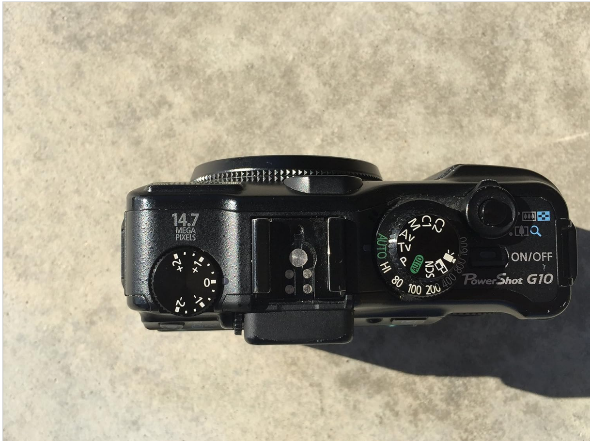
Image: Top view of the Canon PowerShot G10 camera. This image highlights the mode dial, shutter button, and exposure compensation dial, which are crucial for adjusting shooting settings.
