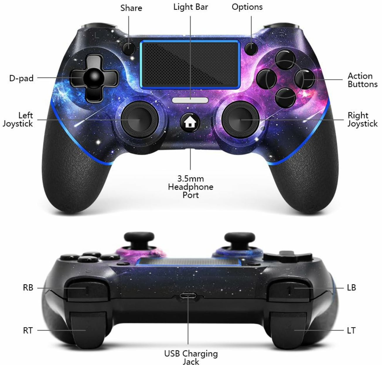
Figure 5: Controller Layout and Button Functions Familiarize yourself with the controller's layout:
