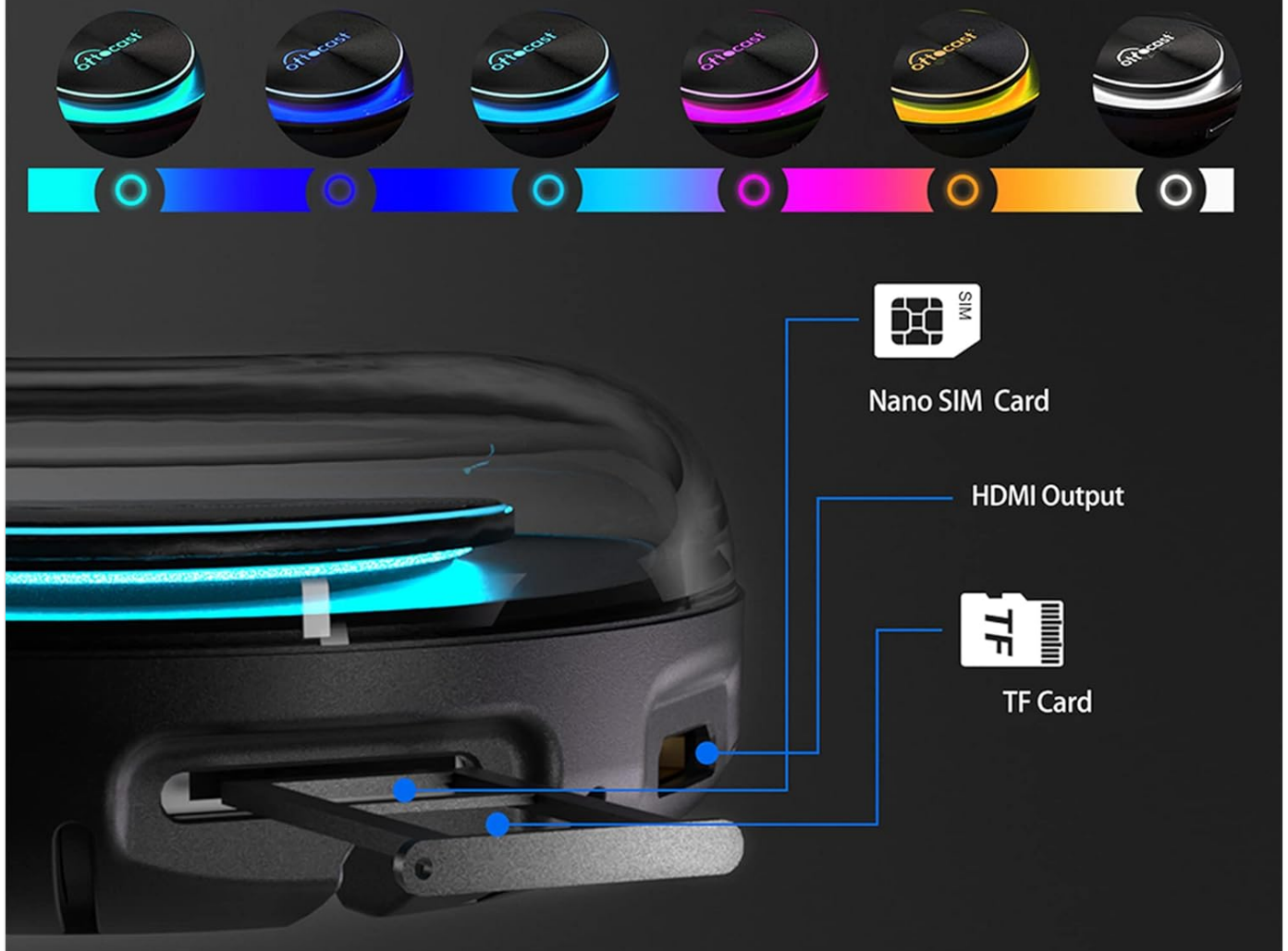
Figure 3.2: Device Ports and Customizable LED Lighting. This image illustrates the side of the OTTOCAST PICASOU 2 device, showing the Nano SIM card slot, TF (microSD) card slot, and HDMI output port. It also highlights the customizable LED ambient light feature, displaying various color options.
