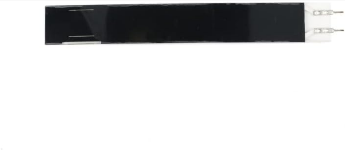
Figure 2.3: Close-up view of the connection pins on the JESSINIE RP-L Film Pressure Sensor, ready for integration into a circuit.
