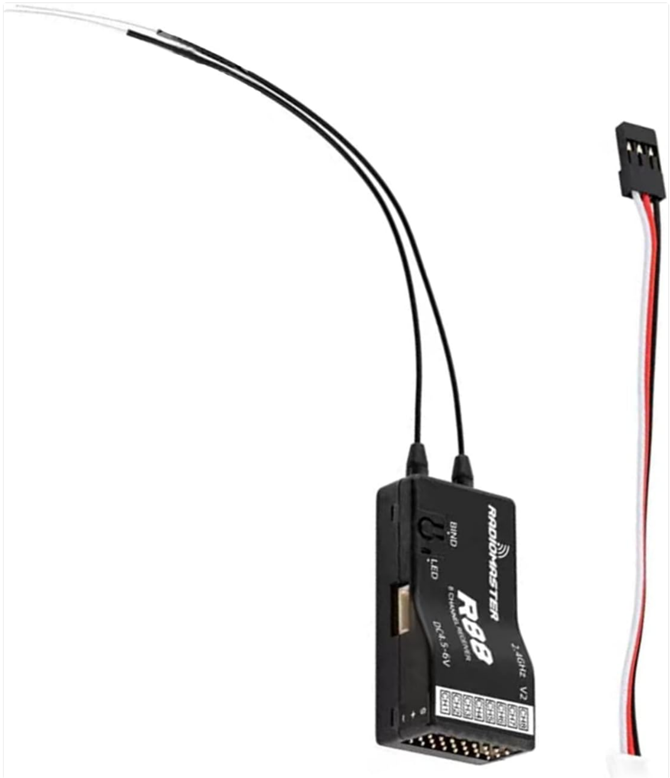
Image: The TECKEEN R88 receiver shown with a standard servo cable connected to one of its PWM output ports, illustrating the connection method.
