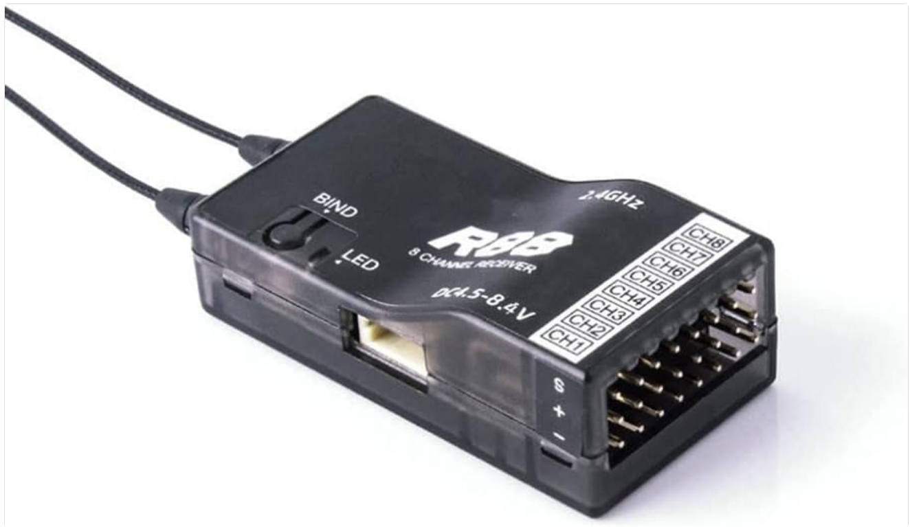
Image: A close-up view of the TECKEEN R88 receiver, highlighting the 'BIND' button, LED indicator, and the 8 PWM channel output ports labeled CH1 through CH8. The power input range DC4.5-8.4V is also visible.
