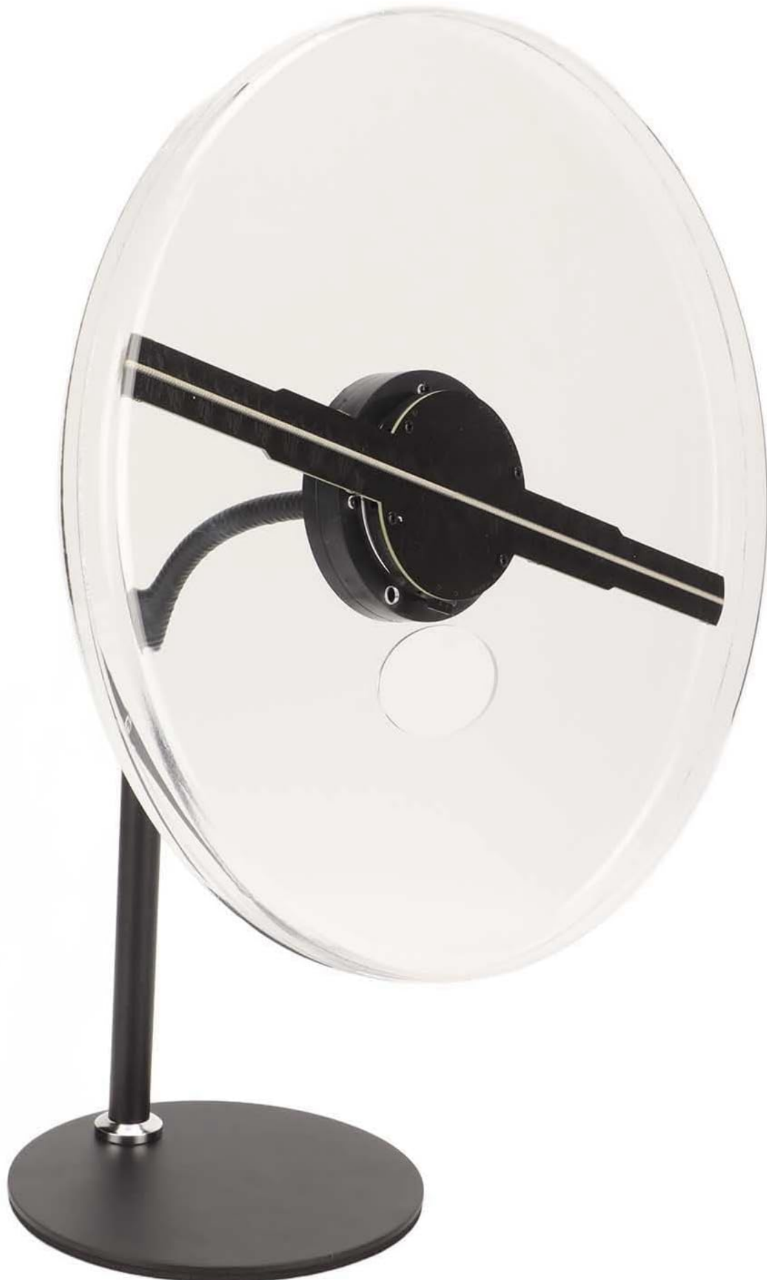
Image: A side profile of the ASHATA F30 Holographic Projector, clearly showing its circular display area and indicating a diameter of approximately 30cm.
