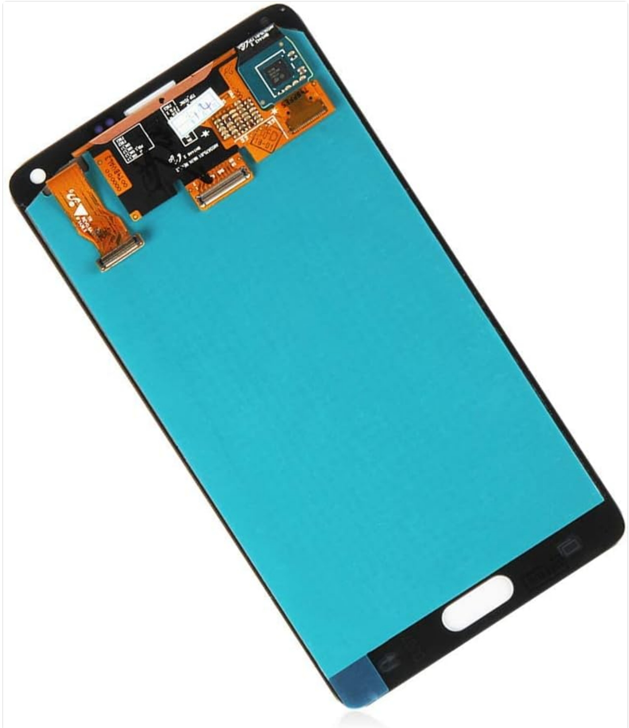
Image: The reverse side of the LCD display assembly, showing the delicate flex cables and connectors that need to be carefully attached to the phone's motherboard during the pre-installation test and final assembly.
