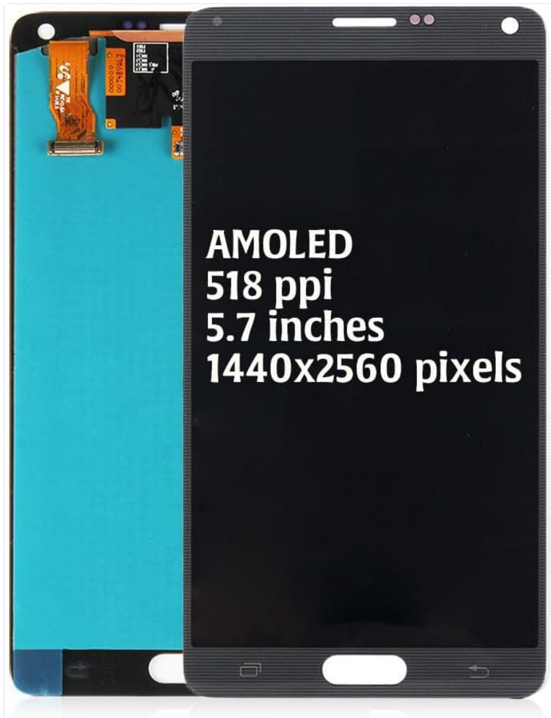
Image: The replacement AMOLED display for Samsung Galaxy Note 4, highlighting key specifications such as 518 ppi, 5.7 inches, and 1440x2560 pixels resolution.
