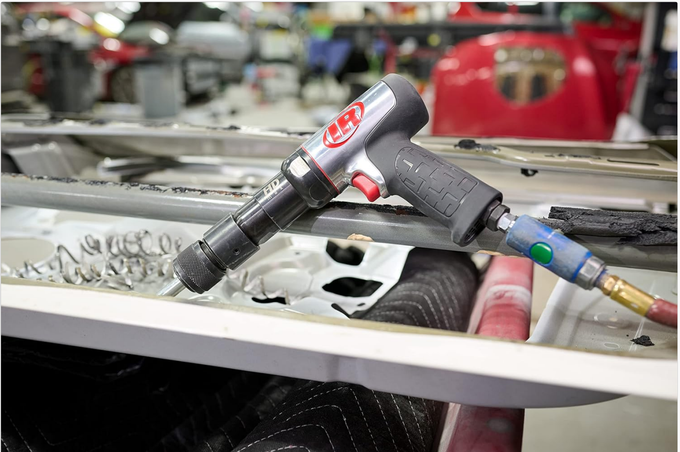
Figure 3: An operator demonstrating the use of the 135MAX Air Hammer for automotive work, showcasing its application in a professional setting.
