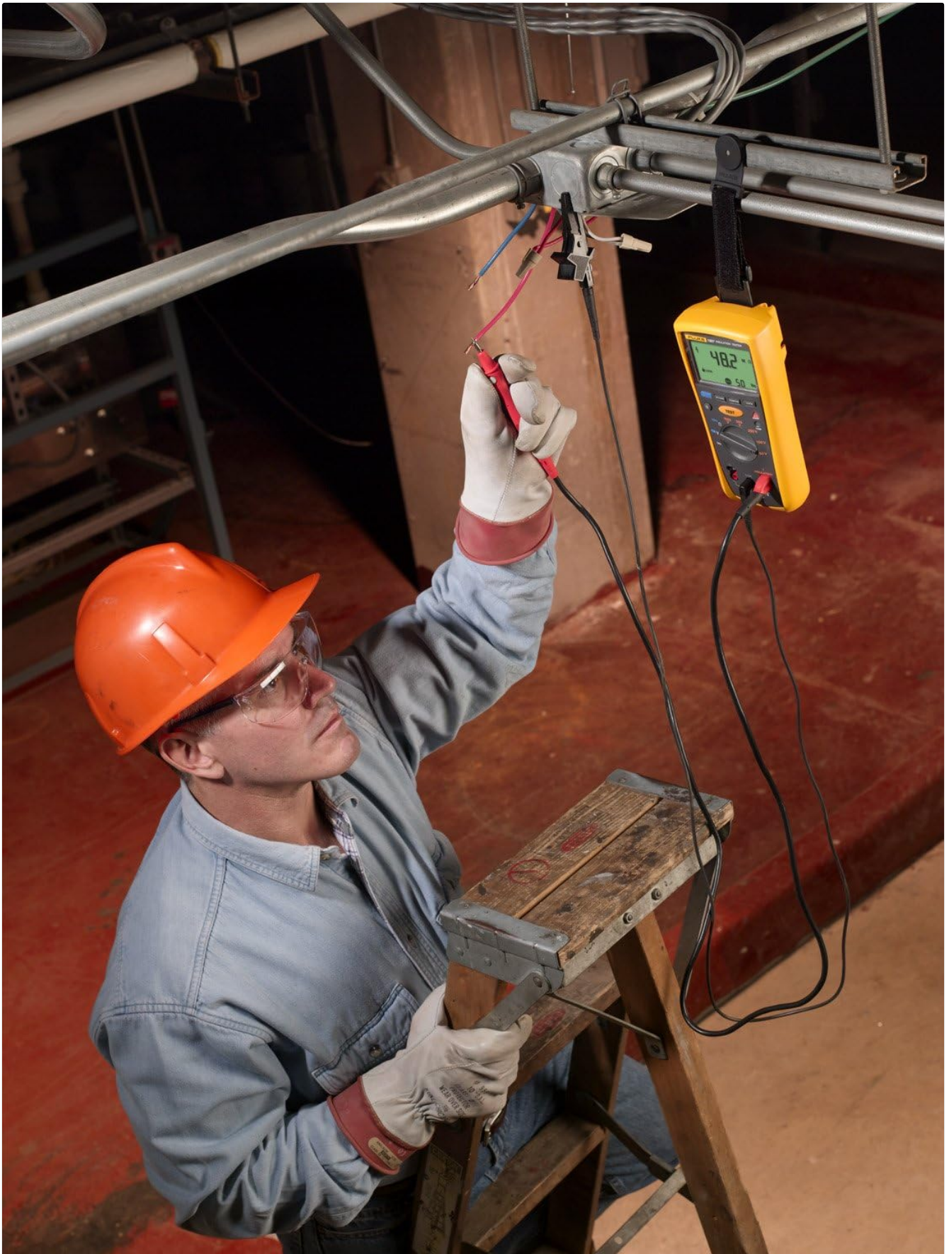
Figure 5.4: A technician utilizing the optional magnetic hanging system with the Fluke 1507, allowing for hands-free operation during overhead electrical work.
