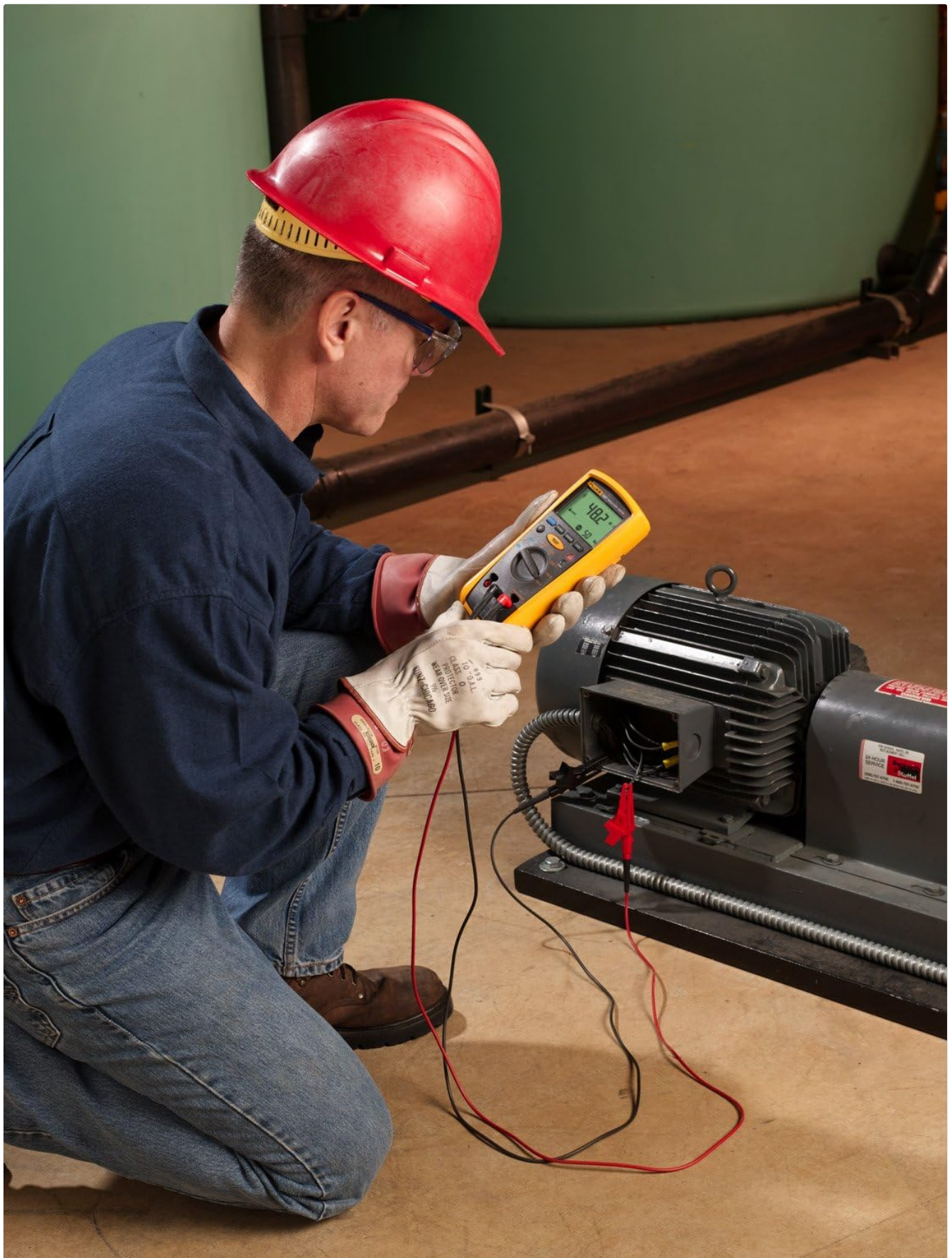
Figure 5.3: A technician performing an insulation test on an industrial motor using the Fluke 1507, highlighting its application in preventative maintenance.
