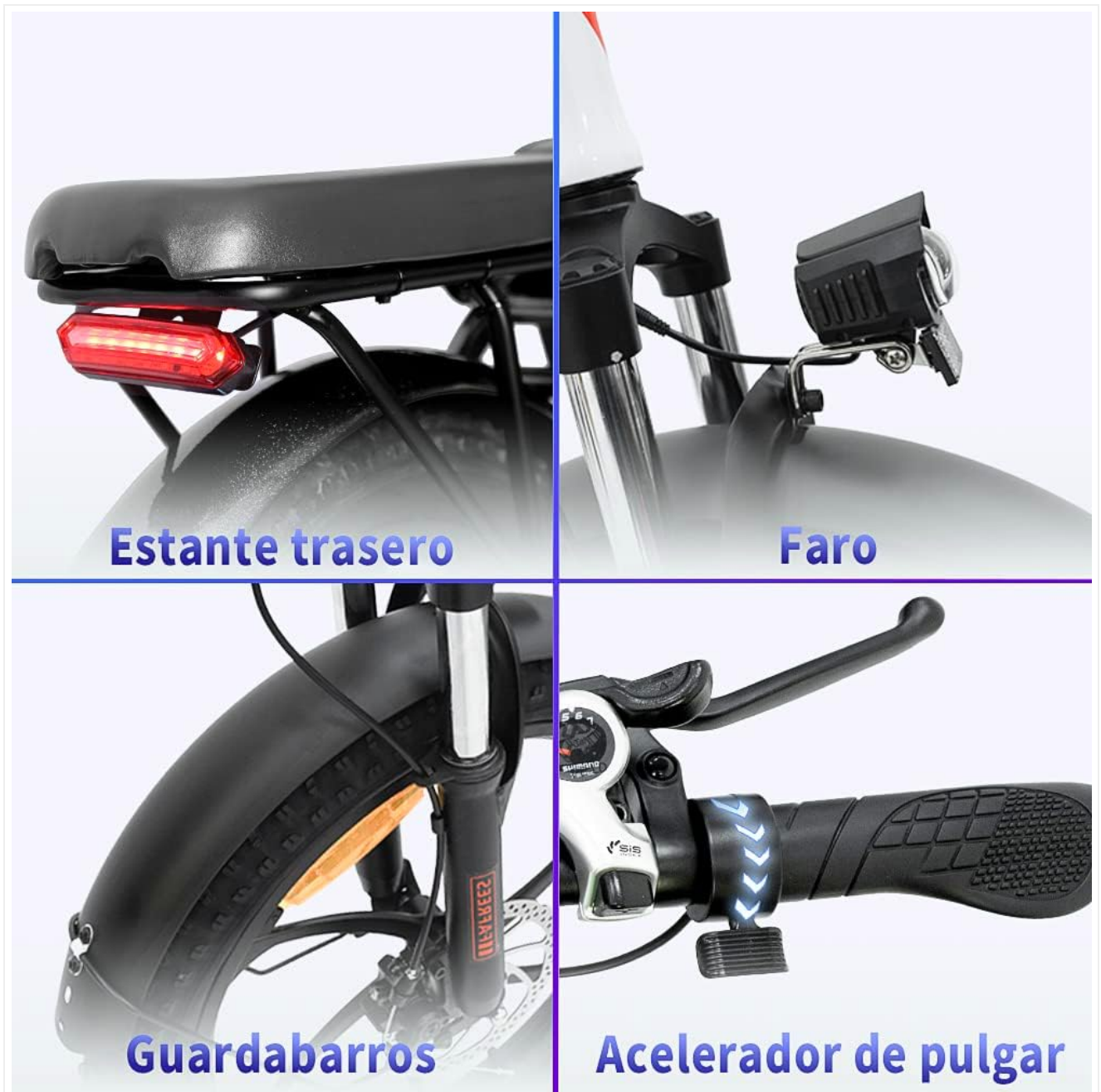
Image: Overview of key components including the rear rack, headlight, fender, and thumb throttle, which controls the full electric mode.
