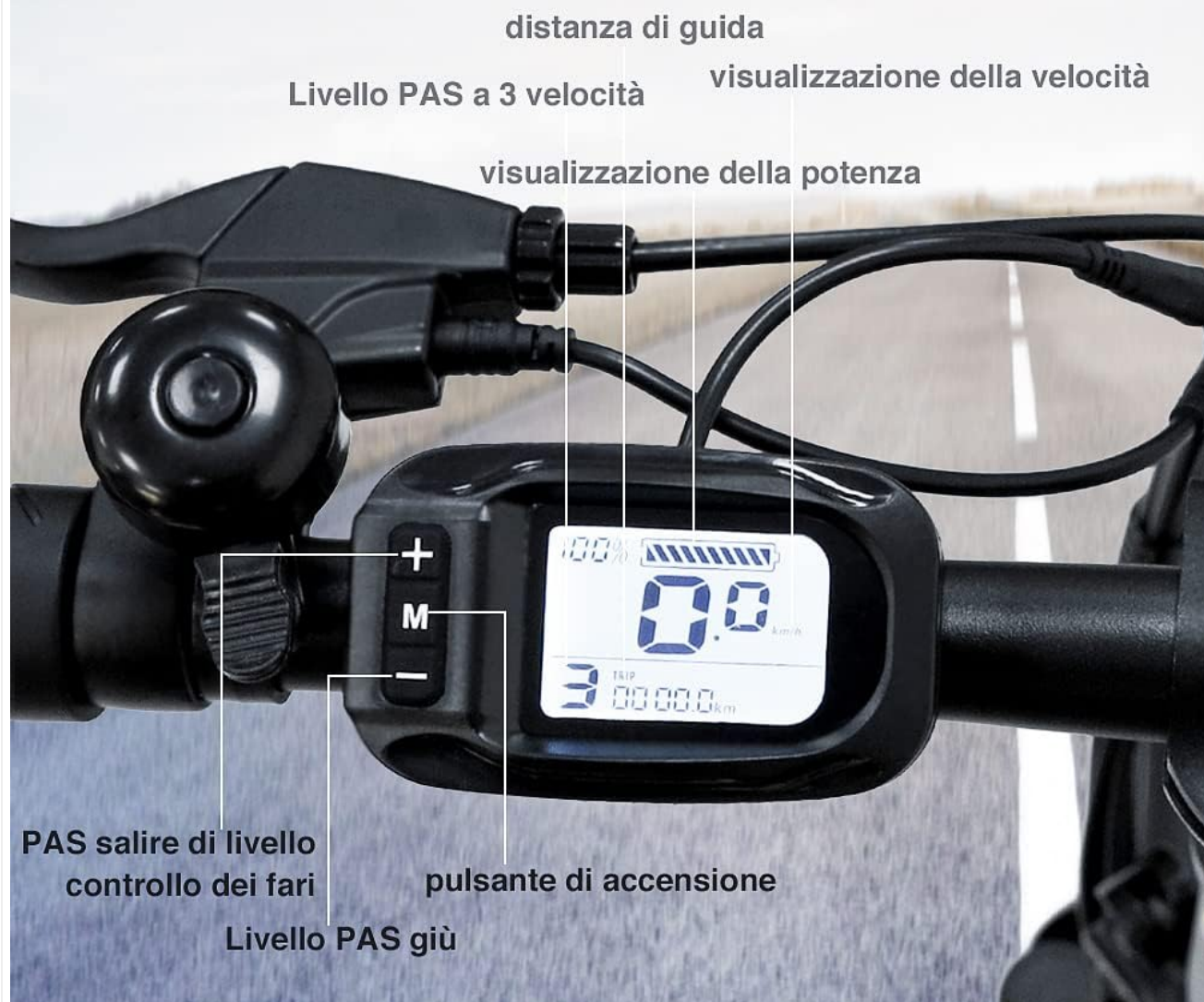
Image: Close-up of the intelligent multifunction display on the handlebar, showing speed, battery, and PAS level indicators, along with control buttons.
