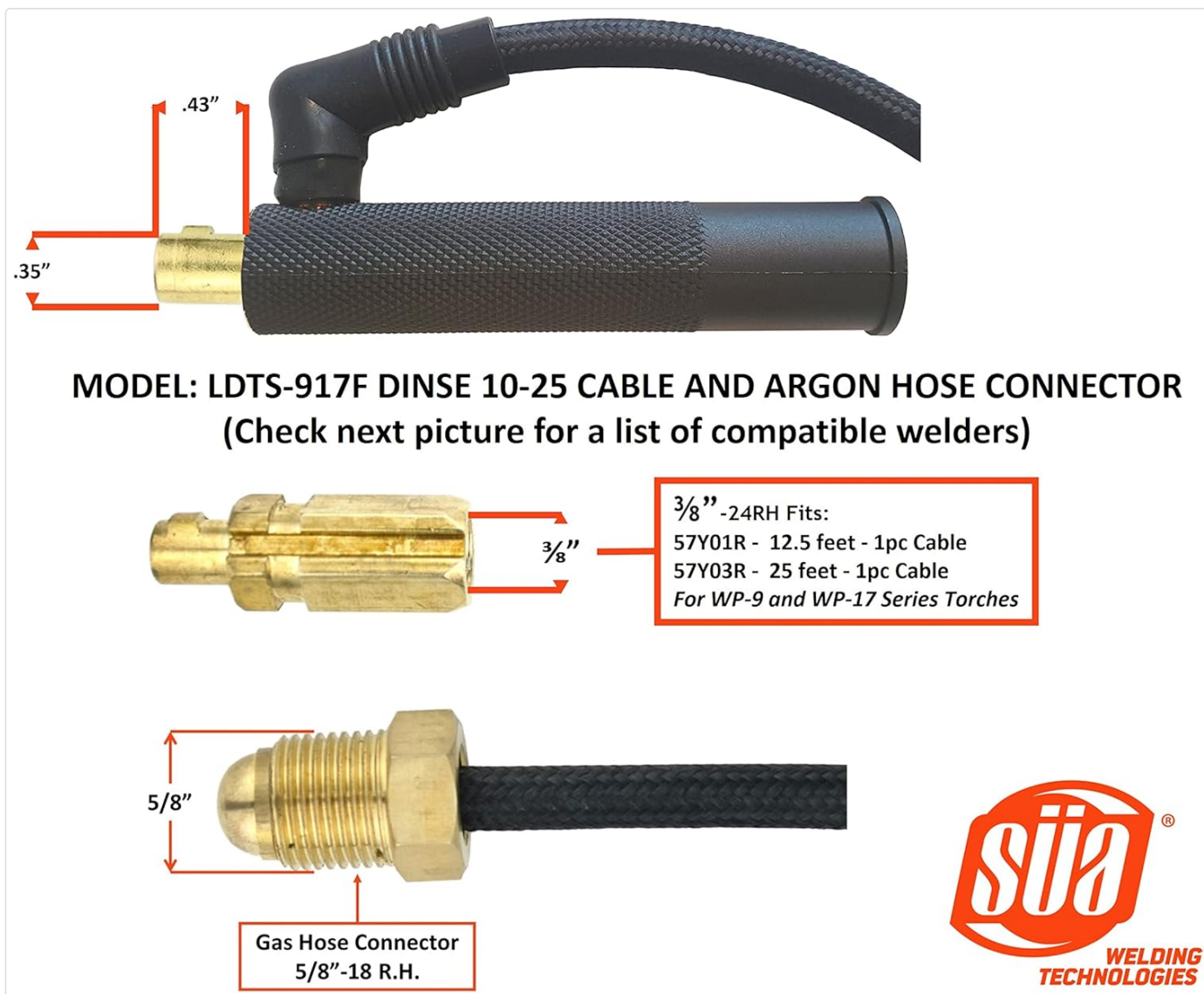
Figure 3.1: Detailed dimensions of the Dinse 10-25 connector and the 5/8"-18 RH gas hose fitting. Also shows compatibility with 57Y01R and 57Y03R 1pc cables for WP-9 and WP-17 Series Torches.
