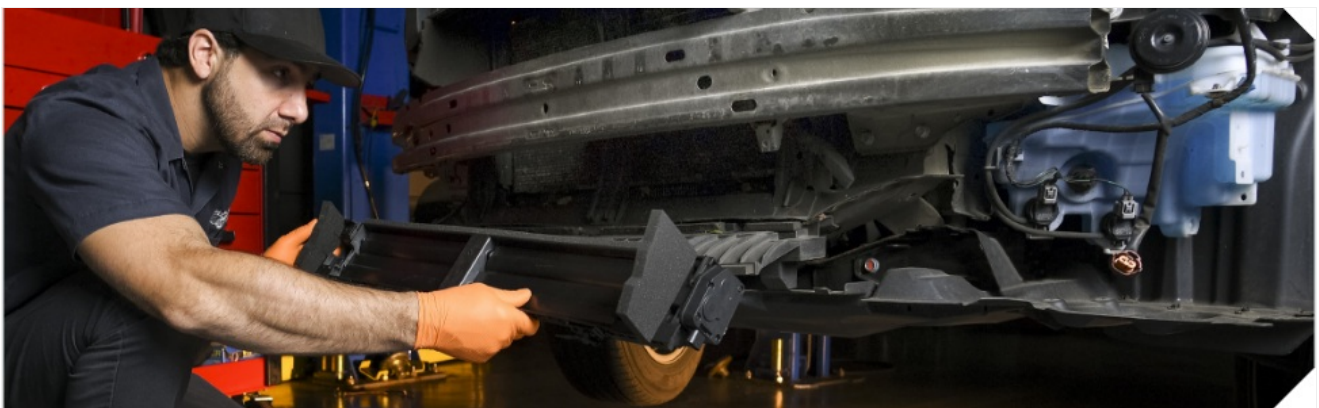
Figure 4.2: A mechanic is shown installing the radiator shutter assembly into the front of a vehicle, illustrating the placement during
