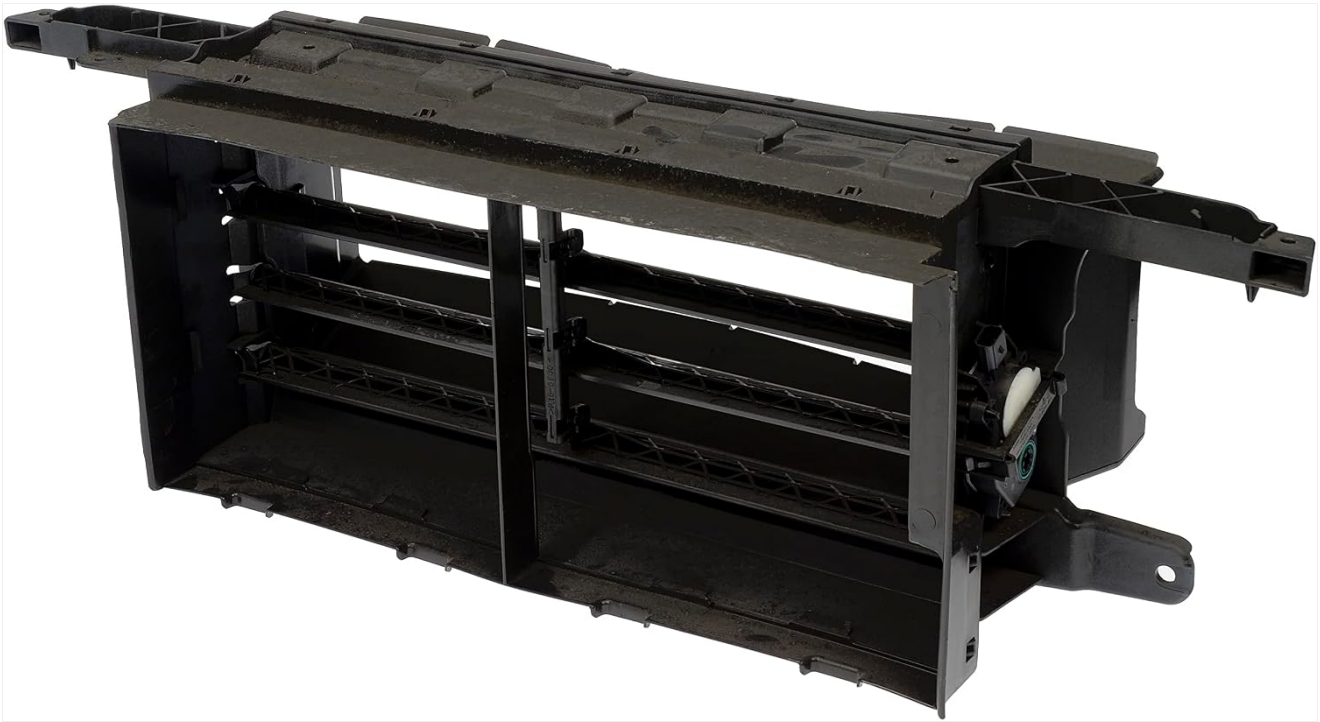
Figure 2.1: Front view of the Dorman 601-392 Radiator Shutter Assembly, showing the main housing and internal louvers.
