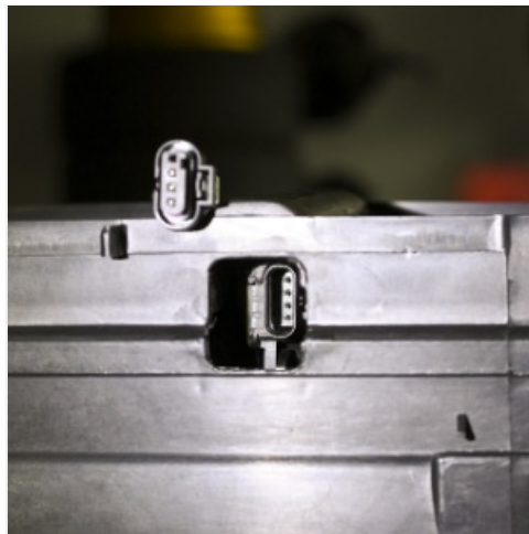
Figure 4.1: Close-up view of the electrical connectors, demonstrating the factory-style connection for the shutter assembly.
