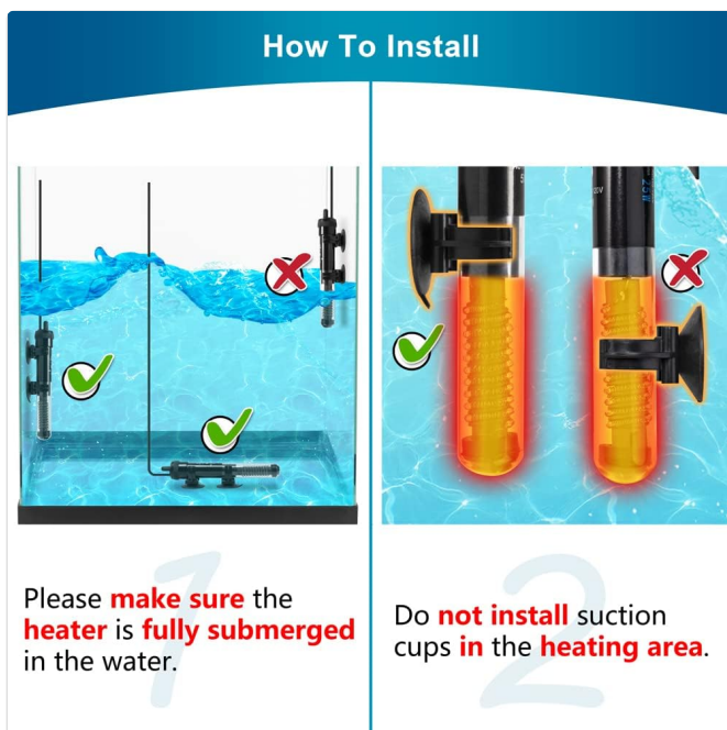
Image: Correct installation showing the heater fully submerged and suction cups placed away from the heating element.
