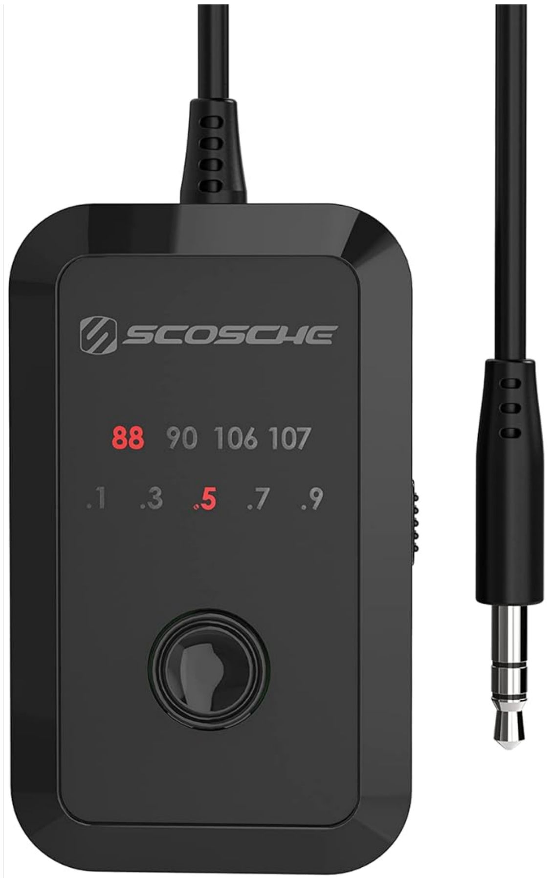
Figure 5: The transmitter's display indicating the selected FM frequency.
