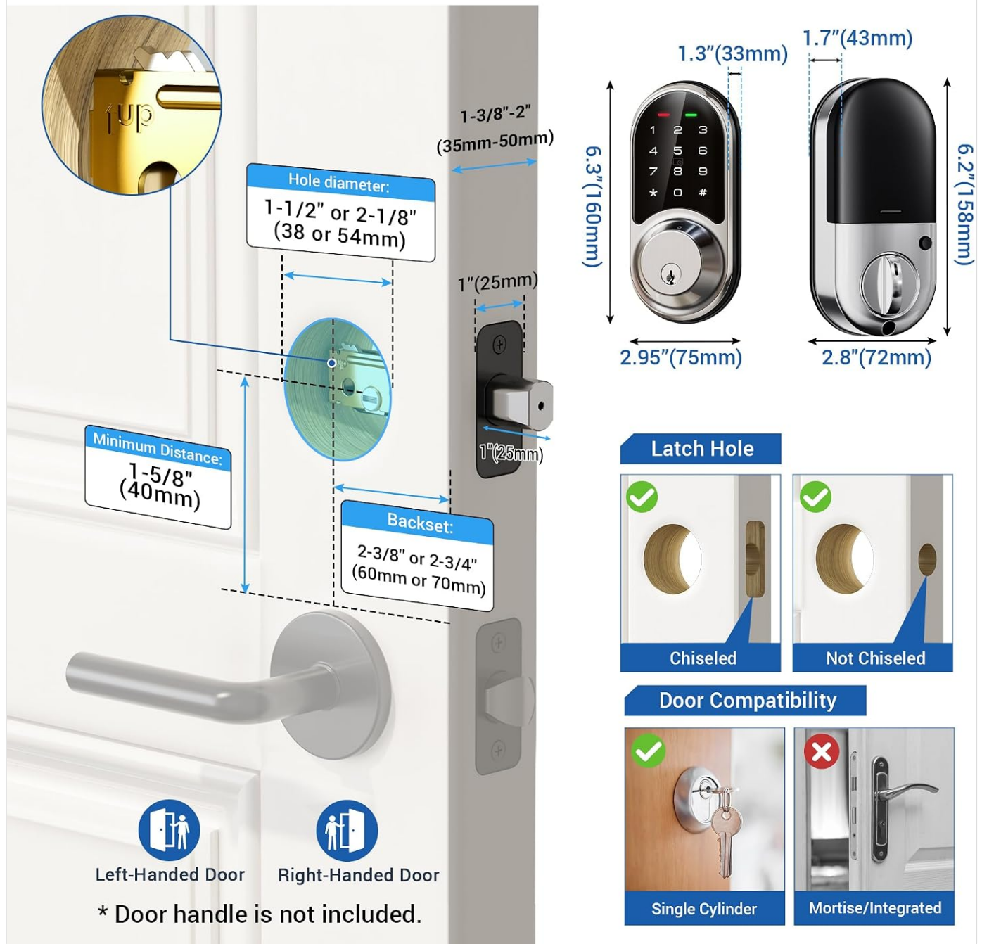
Figure 1: Door Compatibility Diagram. This image illustrates the required door dimensions including hole diameter, backset, and door thickness for proper installation of the Veise RZ06 Smart Lock. It also shows compatibility for left-handed and right-handed doors, and single cylinder deadbolts.
