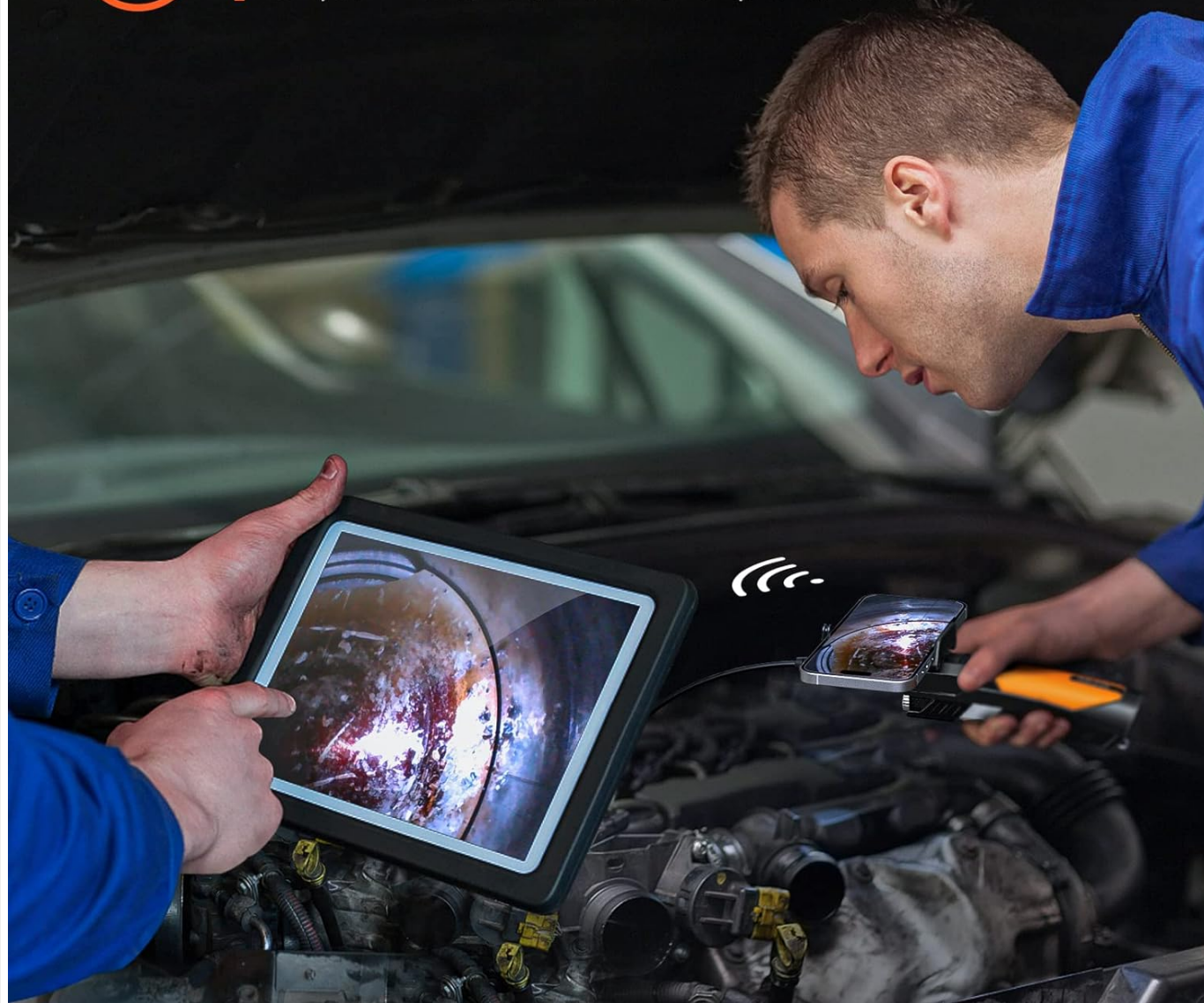
Figure 6.2: View the inspection feed on your iPhone, iPad, or Android smartphone/tablet.
