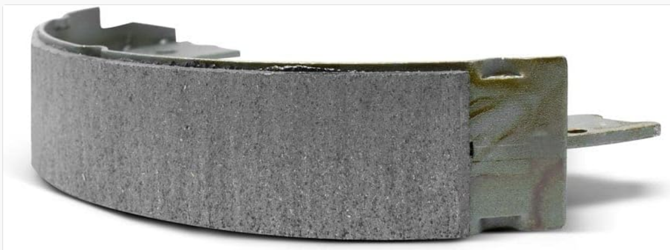
Figure 3: Side profile of a brake shoe, highlighting the friction material. Regular inspection of this lining is vital.
