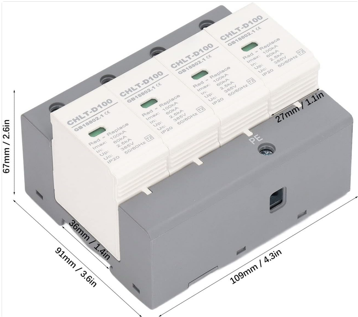
Figure 4.1: Dimensional drawing of the Tyenaza CHLT-D100, showing measurements for installation planning.
