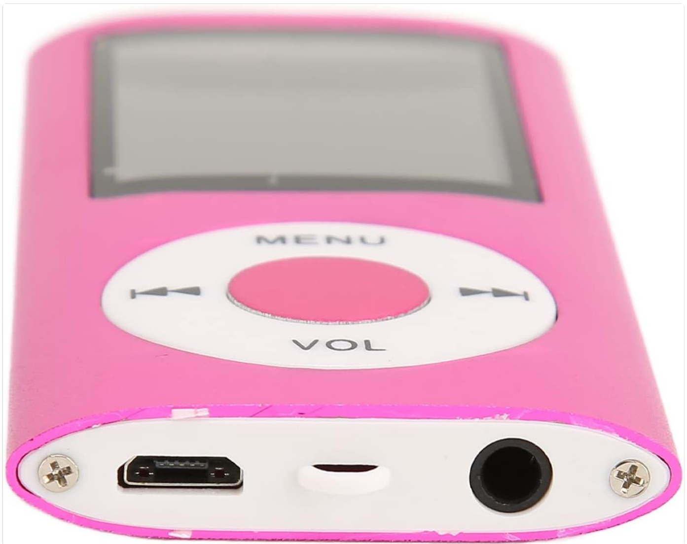
Figure 3.1: Close-up of the player's bottom, illustrating the charging port, memory card slot, and headphone jack.
