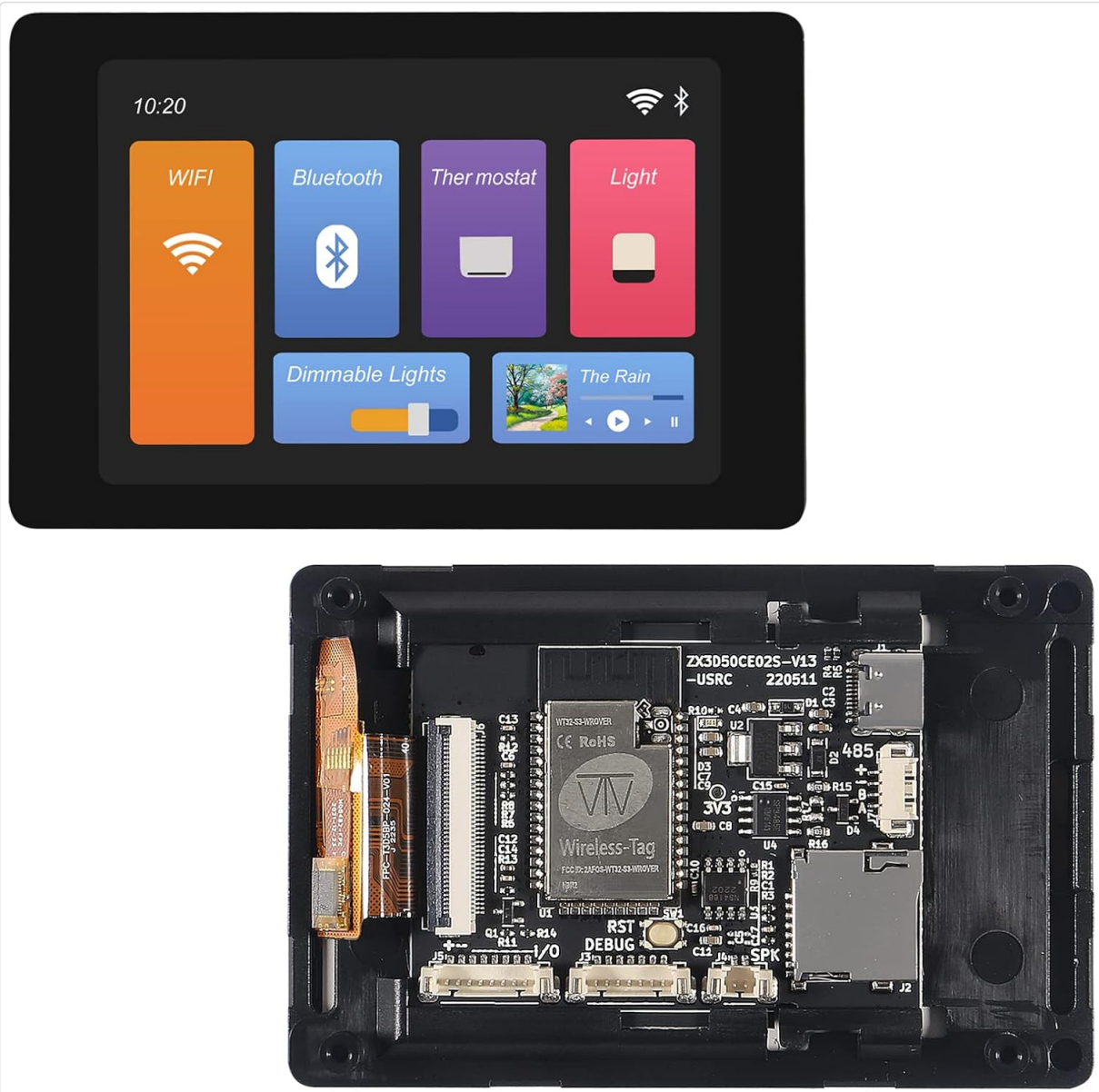
Image 2: Rear view of the WT32-SC01 Plus board, highlighting the ESP32-WROVER-B module, SD card slot, and various connectors.
