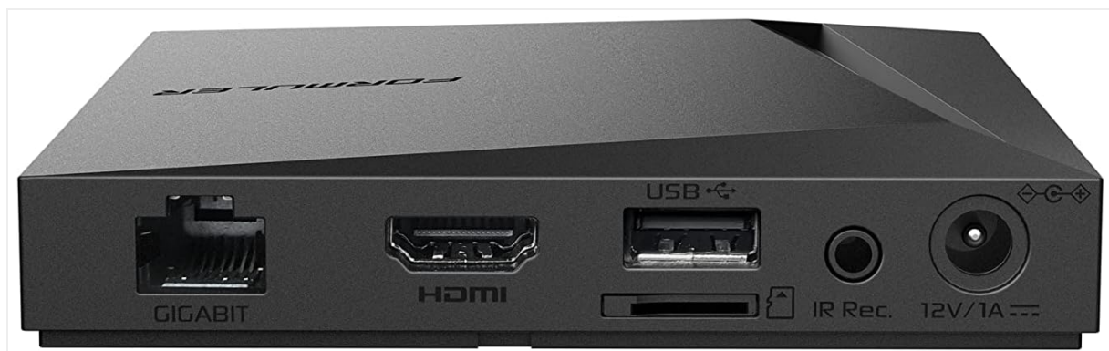
Figure 3.2: Rear view of the Formuler Z11 Pro Max, displaying the Gigabit LAN port, HDMI output, USB 2.0 port, Micro SD Card slot, IR Extension port, and Power Input (12V/1A).
