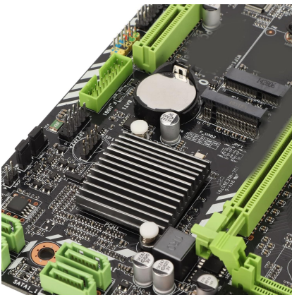
Image 8: A close-up view of the chipset heatsink and the CR2032 button cell battery for the CMOS.
