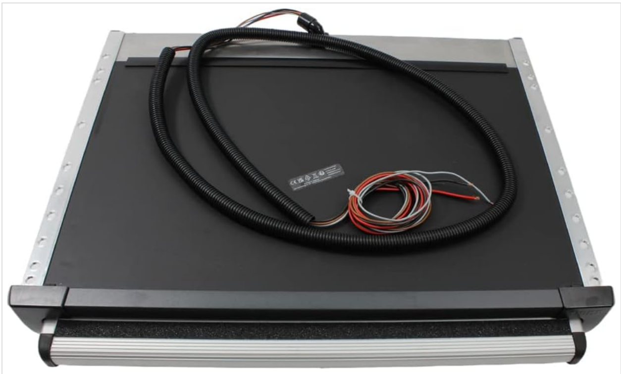
Figure 3: The electric step in its retracted position, showing the integrated wiring.
