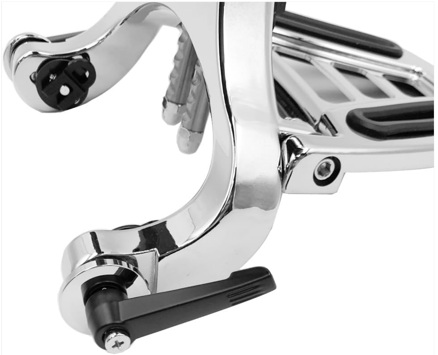
Figure 6.1: Detail of the quick-release lever for adjusting the backrest position.
