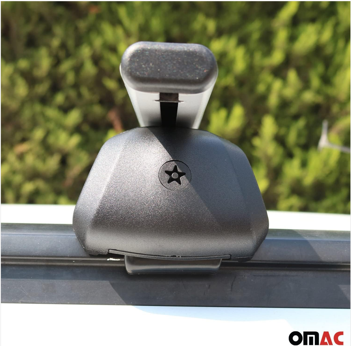
Image 5.3: Using the star wrench to tighten the mounting foot.
