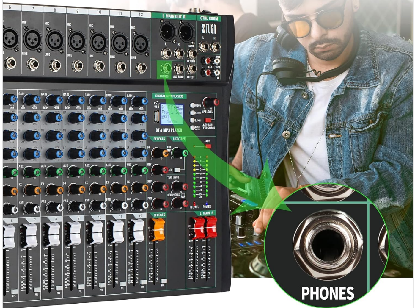
Figure 7: The dedicated headphone output allows for real-time monitoring of the audio mix.
