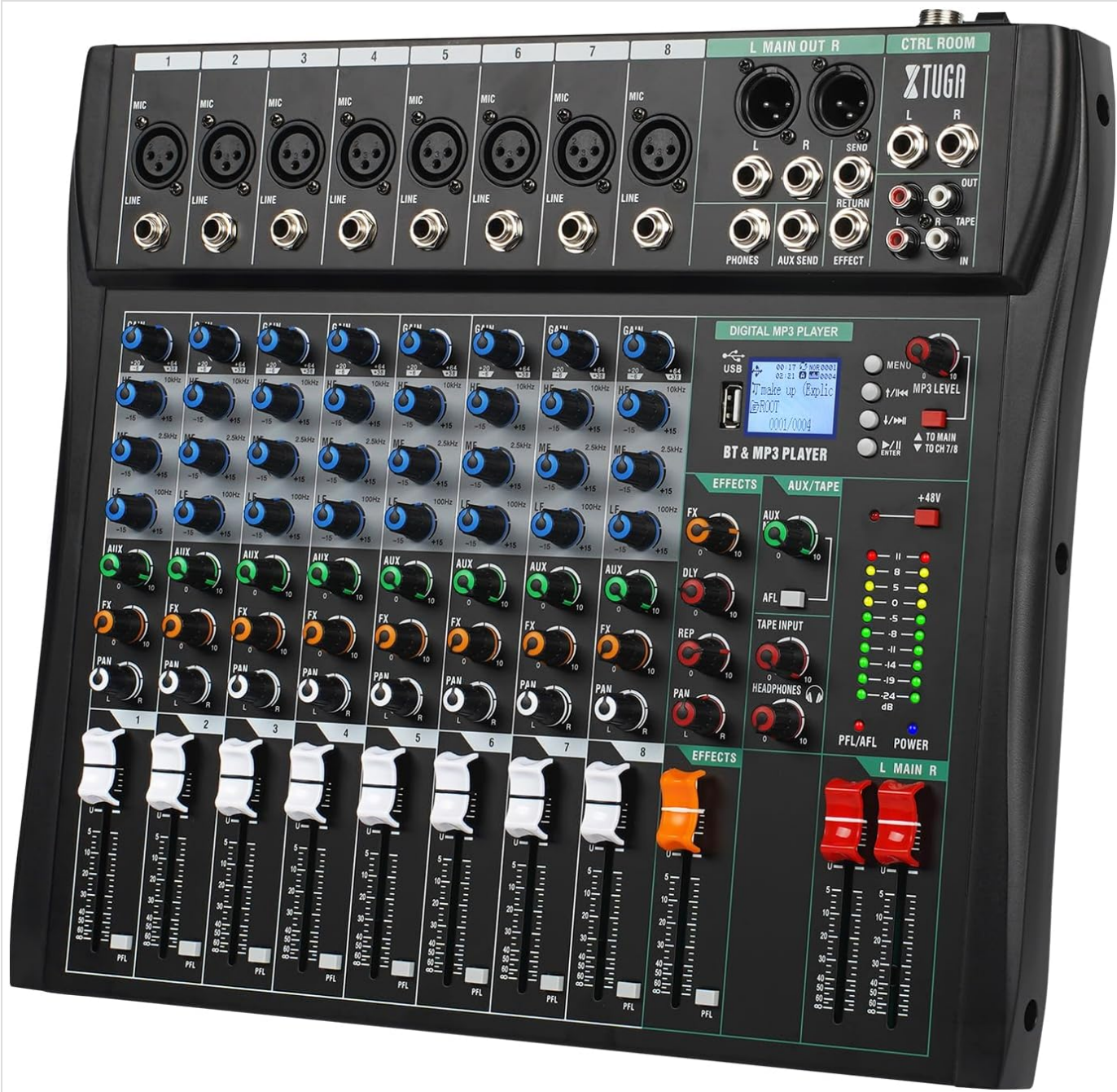
The XTUGA CT80-First Professional Audio Mixer, showcasing its 8 input channels, main output section, and various controls.
