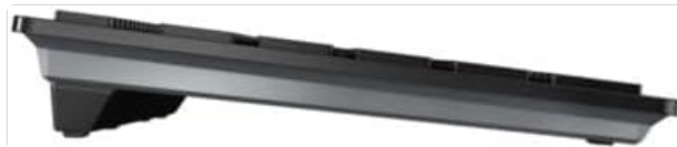
Figure 4.2: Side view of the keyboard demonstrating the elevated angle with the magnetic support bar attached.
