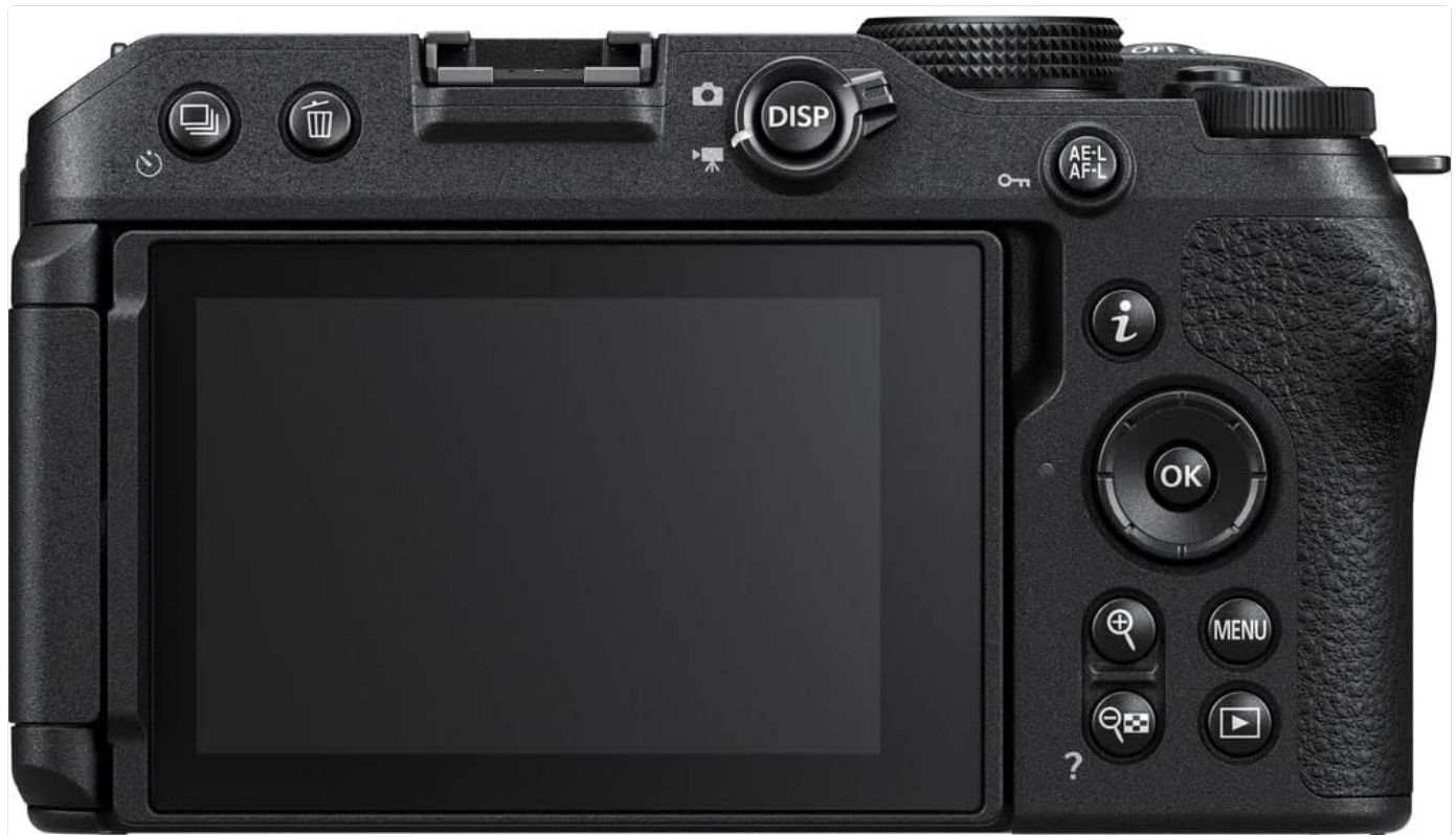
Figure 4: Back view of the Nikon Z30, showing the vari-angle monitor in its closed position.
