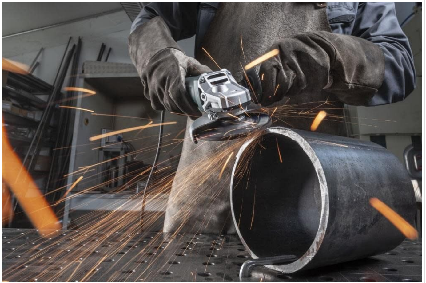
Figure 5.1: Angle grinder in use for cutting metal, demonstrating proper handling and spark direction. The user is wearing protective gear, and sparks are visibly flying away from the operator.
