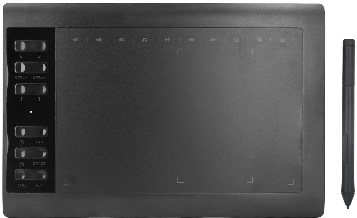
Image: Top view of the Septpenta G10 Graphic Tablet, showing the active drawing area, 12 physical shortcut keys on the left, 10 intelligent shortcut keys on the top, and the passive pen.
