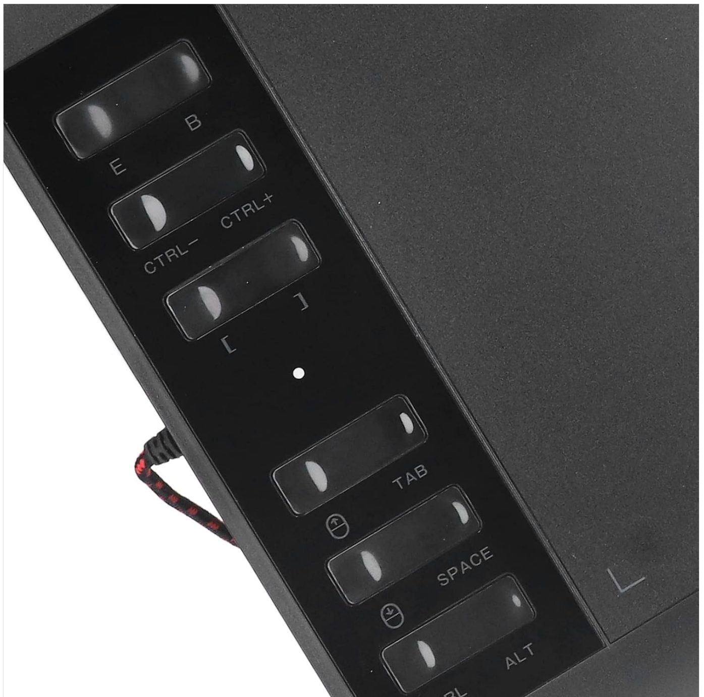
Image: Close-up view of the physical shortcut keys on the left side of the tablet, labeled E, B, CTRL-, CTRL+, brackets, dot, TAB, SPACE, CTRL, and ALT.
