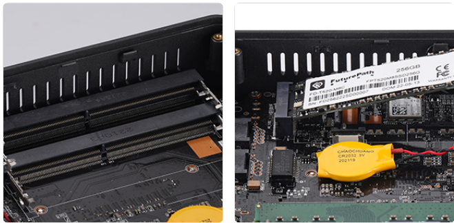
Figure 8: Internal view showing the SO-DIMM DDR5 RAM slots (left) and the M.2 2280 PCIe 4.0 SSD slot (right) for memory and storage upgrades.
