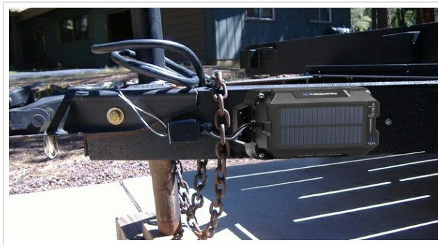
Figure 4: Step 2 - Position the breakaway switch on the trailer drawbar as shown, ensuring proper engagement for the breakaway function.
