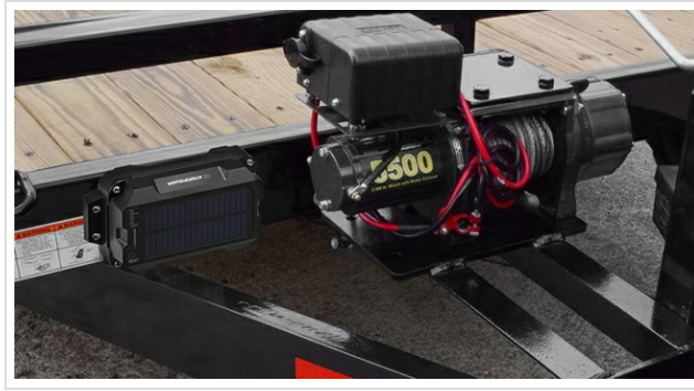
Figure 3: Step 1 - Securely mount the breakaway controller unit to a solid surface on the trailer drawbar, ensuring the solar panel faces upwards for optimal sunlight exposure.
