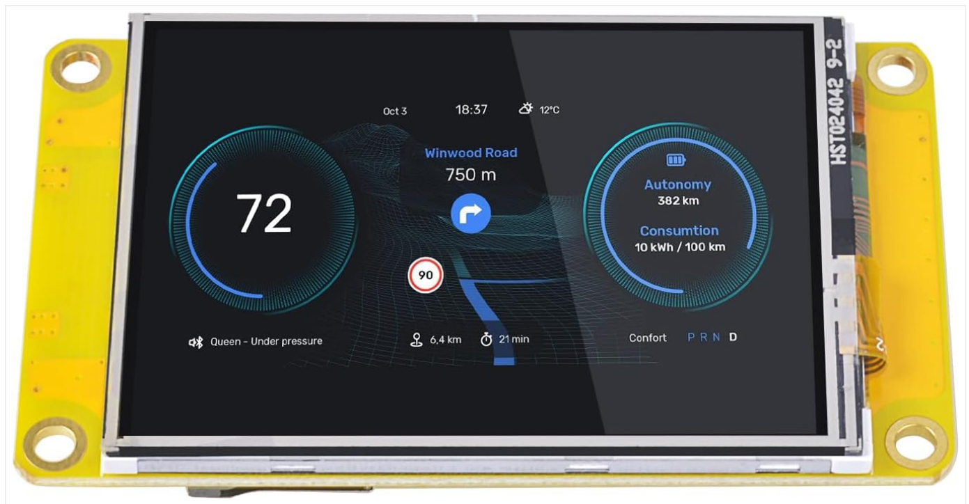
Figure 1.1: Nextion HMI Display 2.4" Discovery Series NX3224F024.
