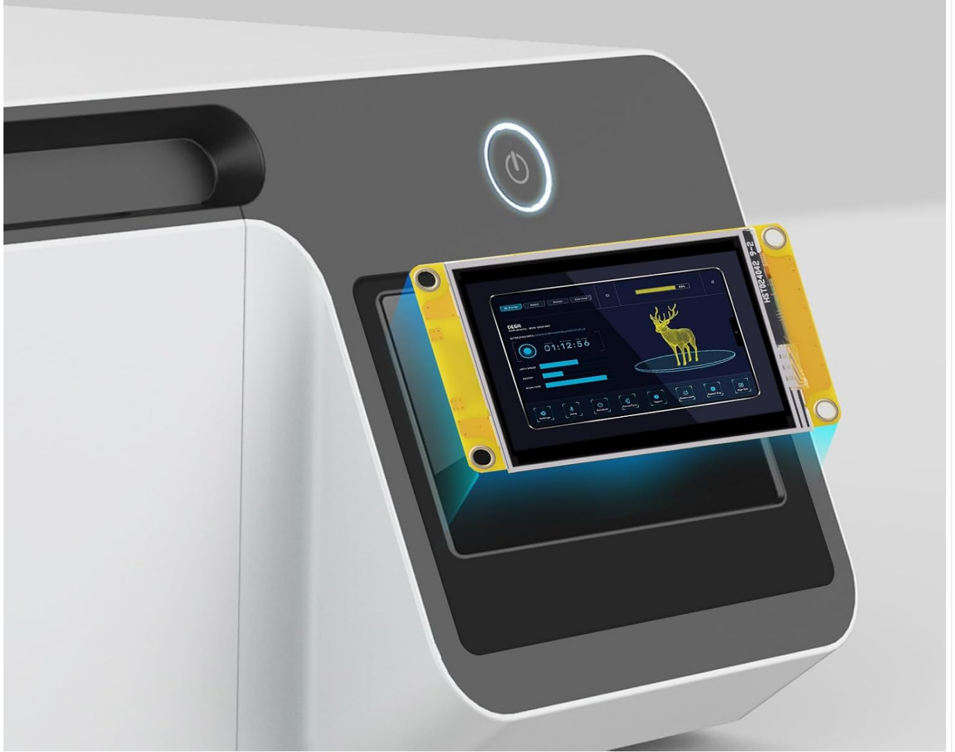
Figure 6.2: The Nextion Display serving as a control interface for a 3D printer, demonstrating its utility in additive manufacturing.
